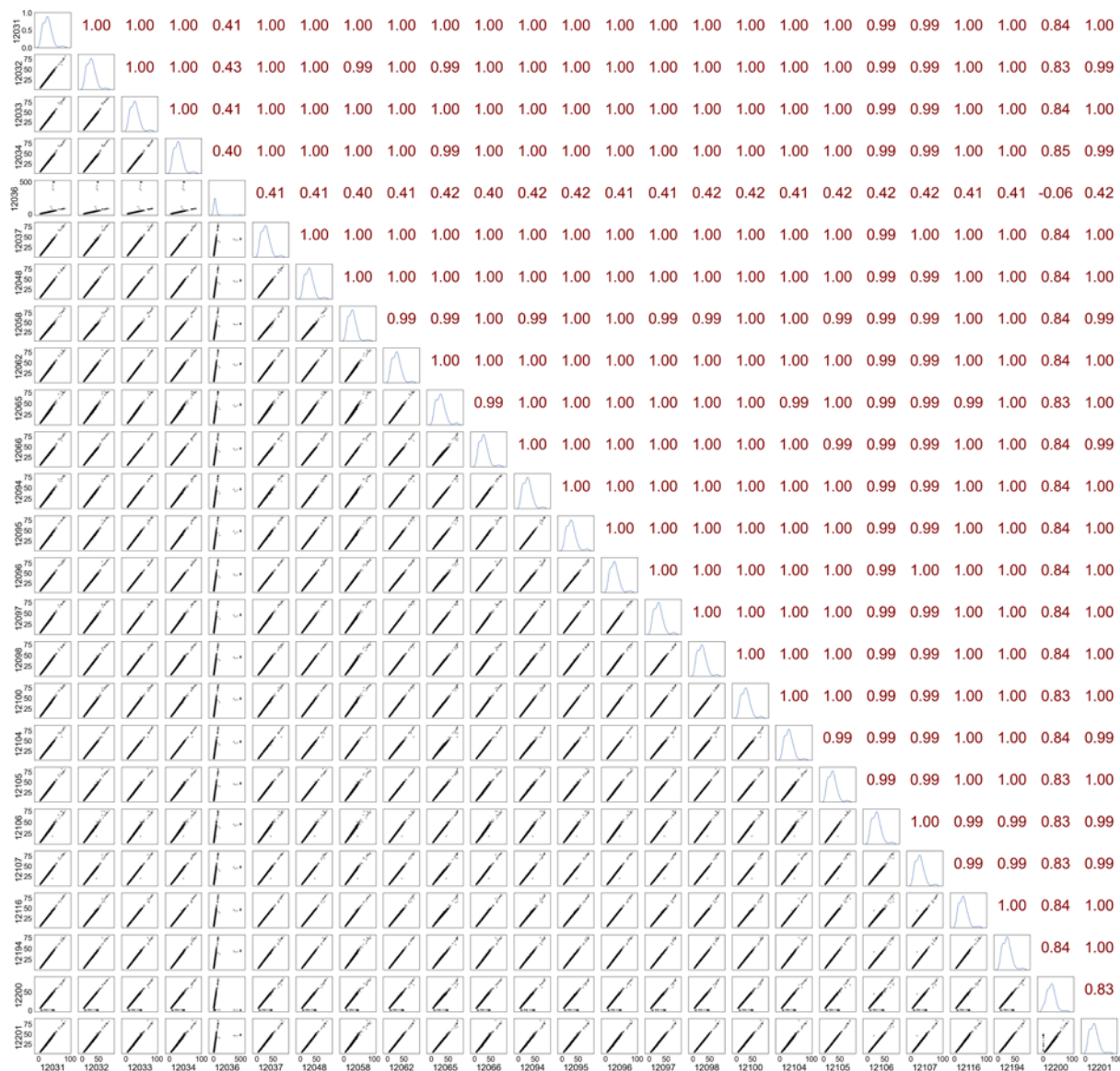
Figure A29: Intra-device correlation for manufacturer-reported data of PM 2.5 from the Aurassure sensor
