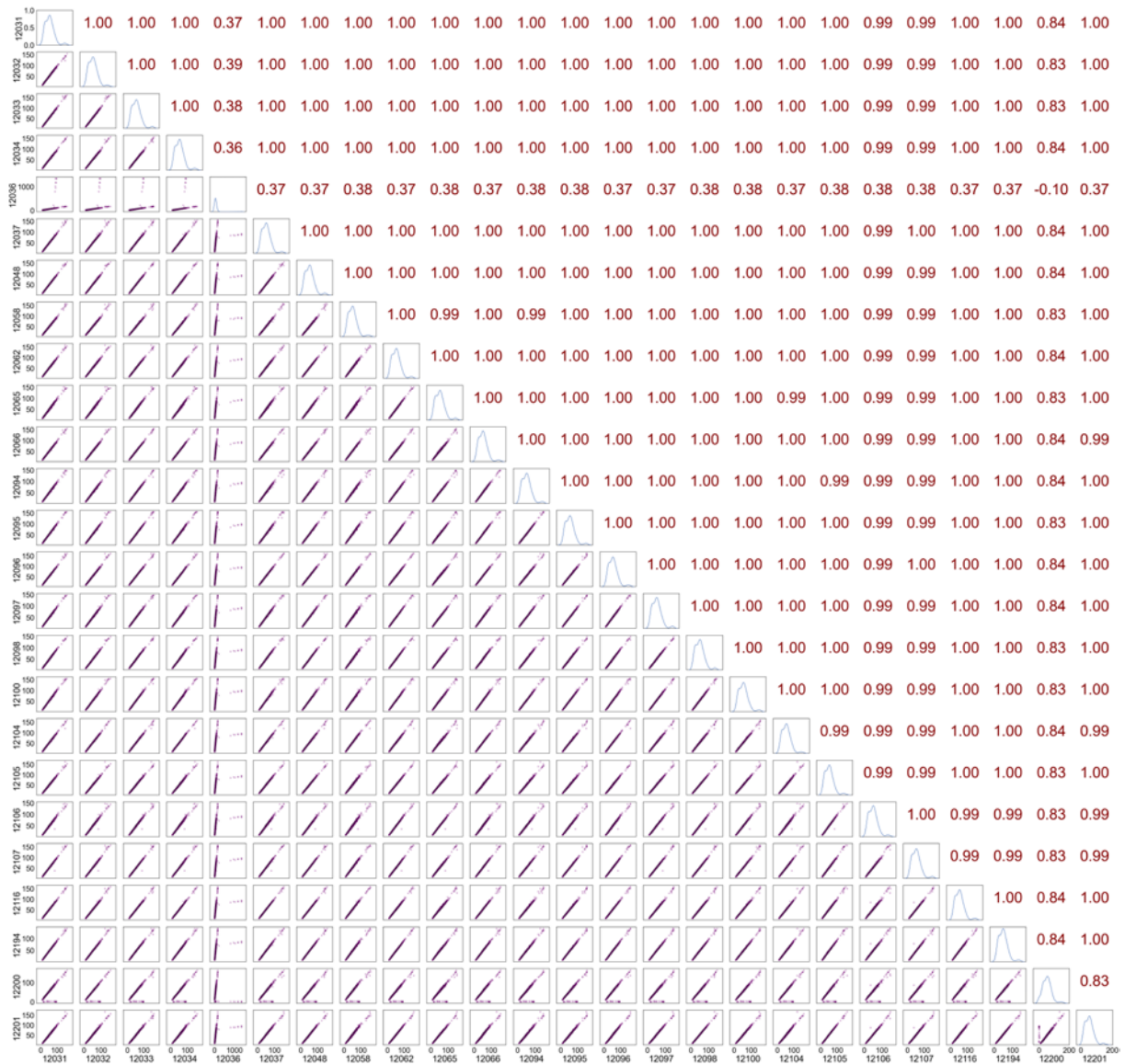
Figure A30: Intra-device correlation for manufacturer-reported data of PM_{10} from the Aurasure sensor
