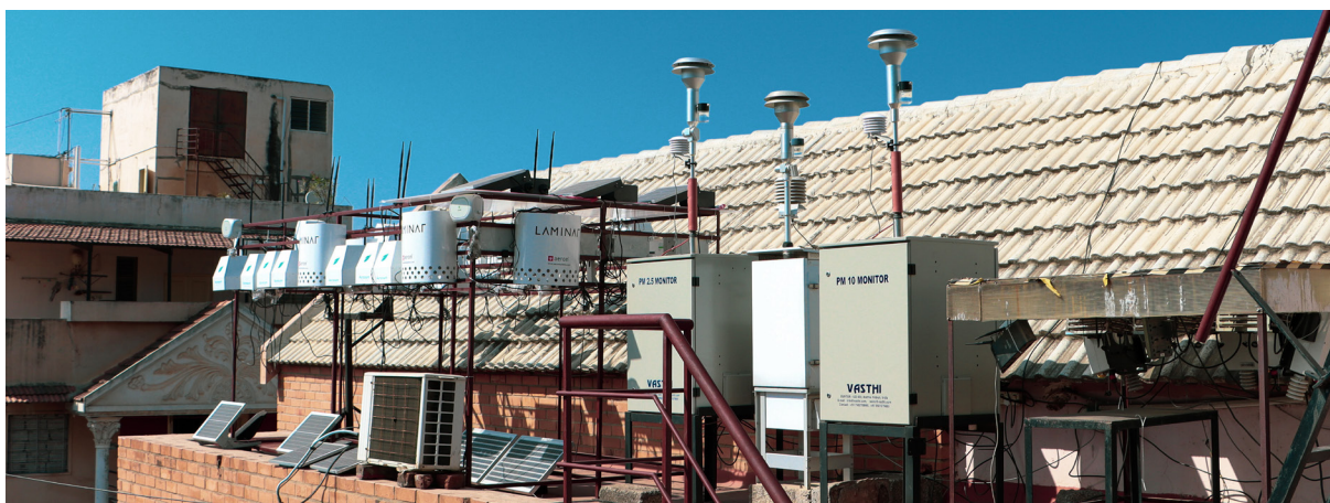
Figure 4: The Indi-SET facility established at the CSTEP campus in Bengaluru. The PM monitors for PM_{2.5} and PM_{10} are placed outdoors in weatherproof enclosures next to the sensor test bed that accommodates up to 60 sensor nodes.
