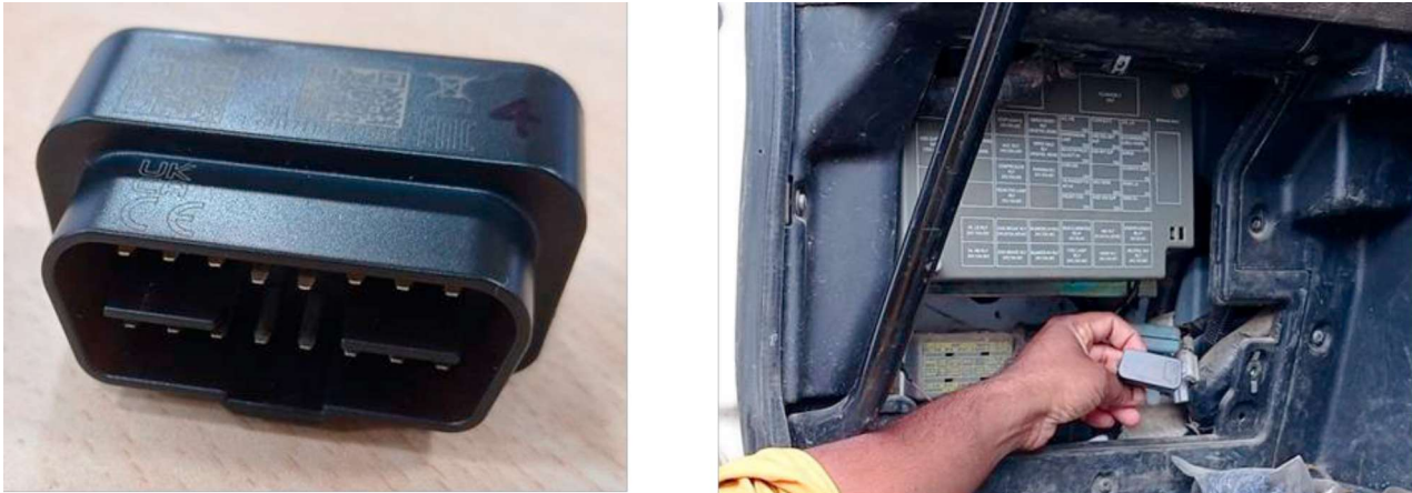
Figure 1: (a) On-board diagnostic (OBD) devices used in the study (left), and (b) an OBD device plugged in the port (right)
