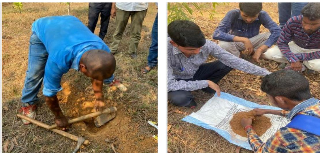
Figure 8: Photographs of the field teams collecting soil samples
