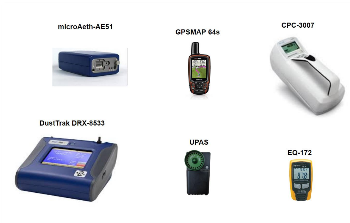
Figure 1: A collage of instruments used for on-road air pollution monitoring (source: tsi.com, garmin.com; aethlabs.com; accsensors.com)
