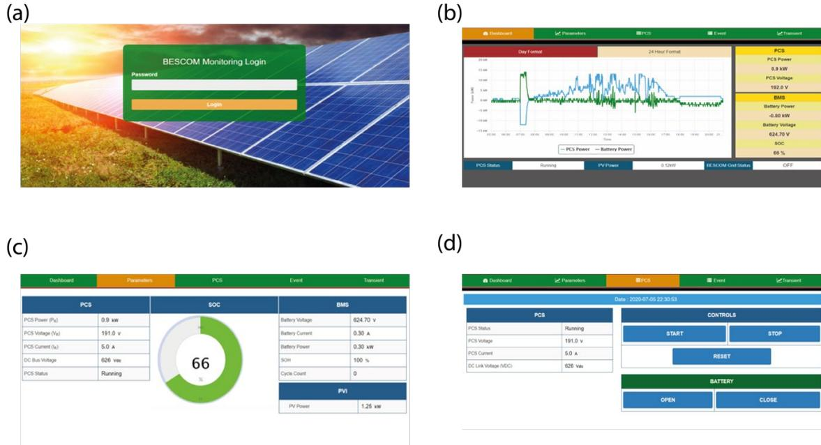
Figure 9: Snapshots of the user interface to the PCS for remote monitoring: (a) the user login page; (b) the dashboard showing the energy profiles related to PV generation, battery energy, and the total PCS energy as a function of time of day; (c) the display of certain parameters related to the PCS power and battery SoC; and (d) certain system-level controls in the same interface
