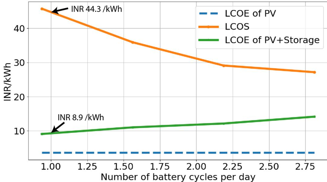
Figure 20: Levelised cost of solar PV plus storage plant along with the same for subcomponents (PV only and storage only) as a function of battery utilisation. The PV plant and storage sizes are maintained constant throughout the calculations. The values highlighted with arrows are used in the analysis in the subsequent sections.
