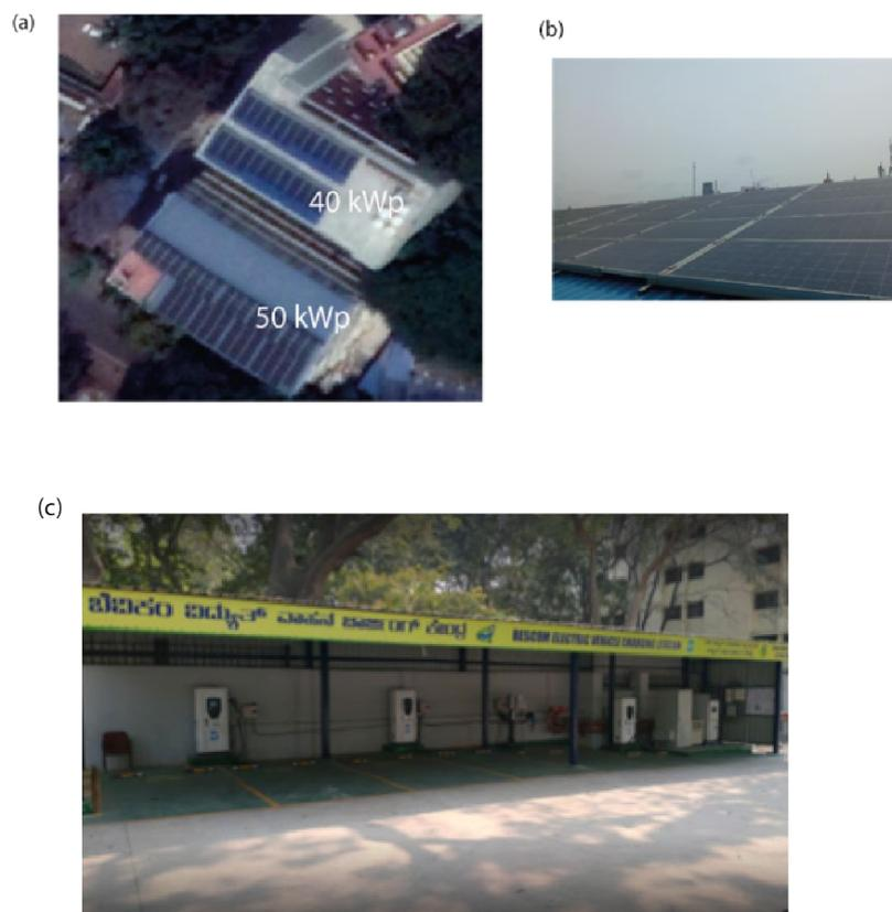
Figure 2: (a) Top view of the BESCO Corporate Office premises in Bengaluru. The solar panels for both the 40 and 50 kWp systems of the two buildings are visible. (b) Enlarged view of the solar panels of the 40 kWp system and (c) EV charging station used for the pilot study
