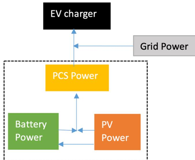
Figure 13: The schematic of the energy/power flow from various components to the EV charger
