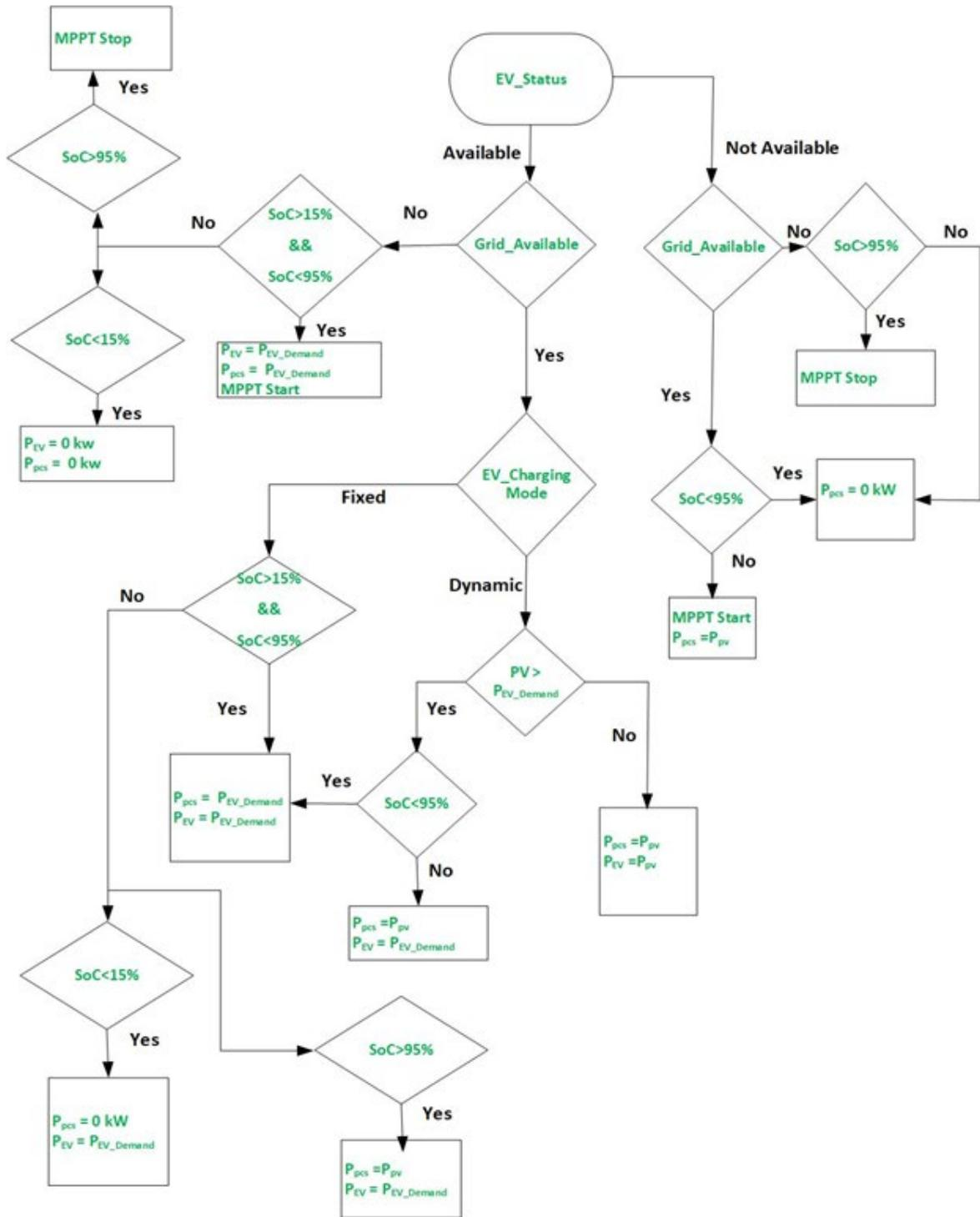
Figure 8: Source prioritisation algorithm for RTPV- and battery-coupled EV charger. Parameters' meaning – SoC: state of charge,  $P_{EV}$ : power demand from the EV,  $P_{PCS}$ : power delivered by the PCS,  $P_{PV}$ : power delivered/generated by the solar panels
