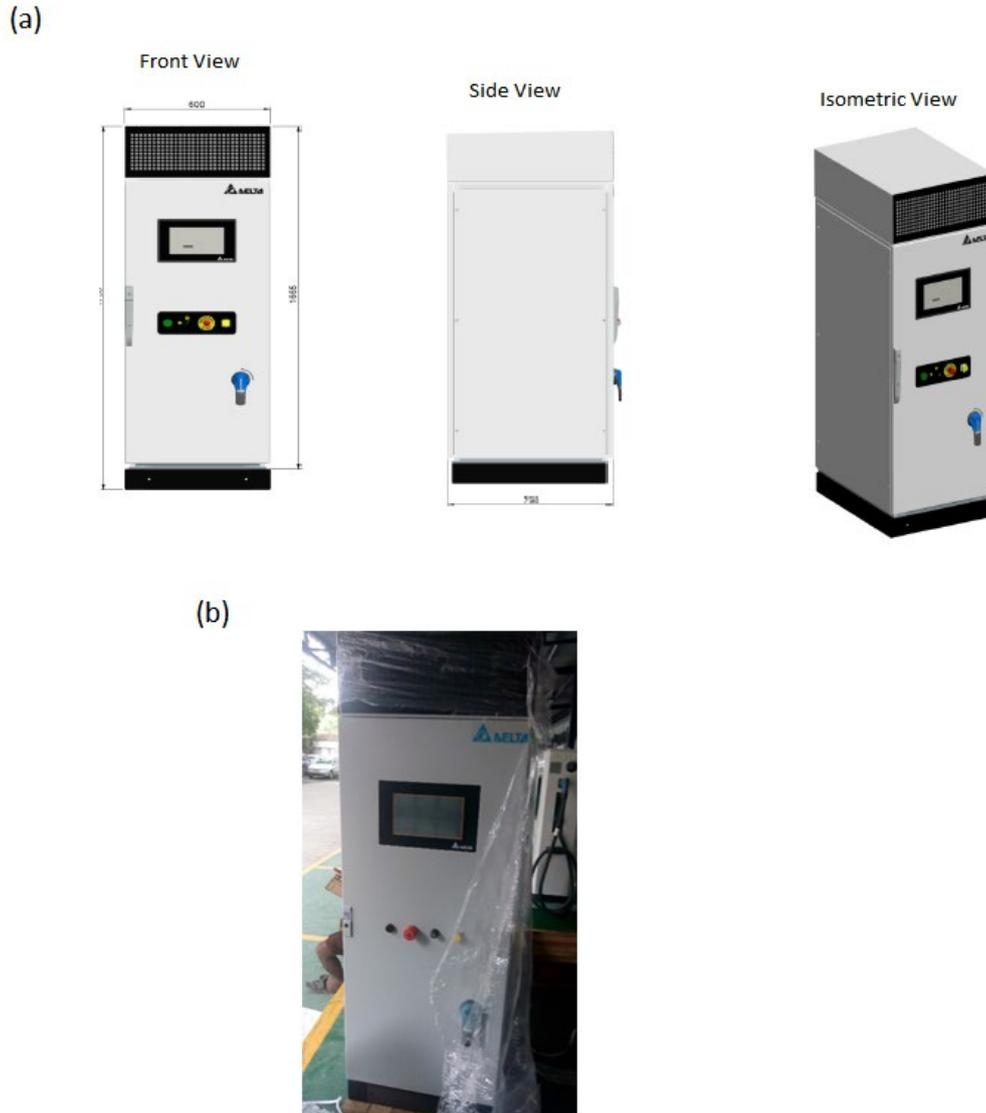
Figure 5: (a) Schematic of the PCS supplied by Delta Electronics and (b) snapshot of the system on-site
