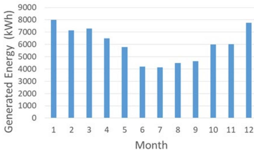
Figure 3: Monthly PV energy generation data from simulation for the 40 kWp RTPV system (for the year 2020)
