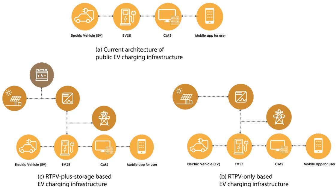
Figure 14: (a) Current system architecture of EV charging station, (b) EV charging with RTPV only, and (c) EV charging station with RTPV plus energy storage system
