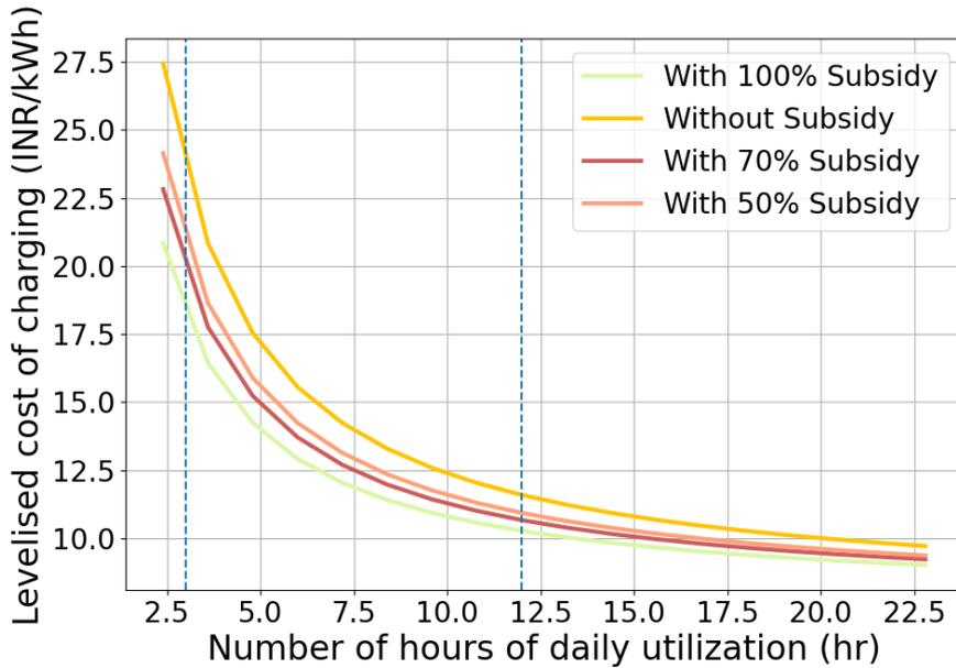
Figure 17: The effect of subsidies on the LCOC at the model EVCS (cost of grid electricity = INR 5/kWh for all cases)
