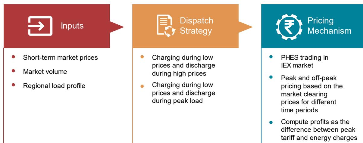
Figure 7: Tariff computation method for energy arbitrage/peak-load shaving/load following
