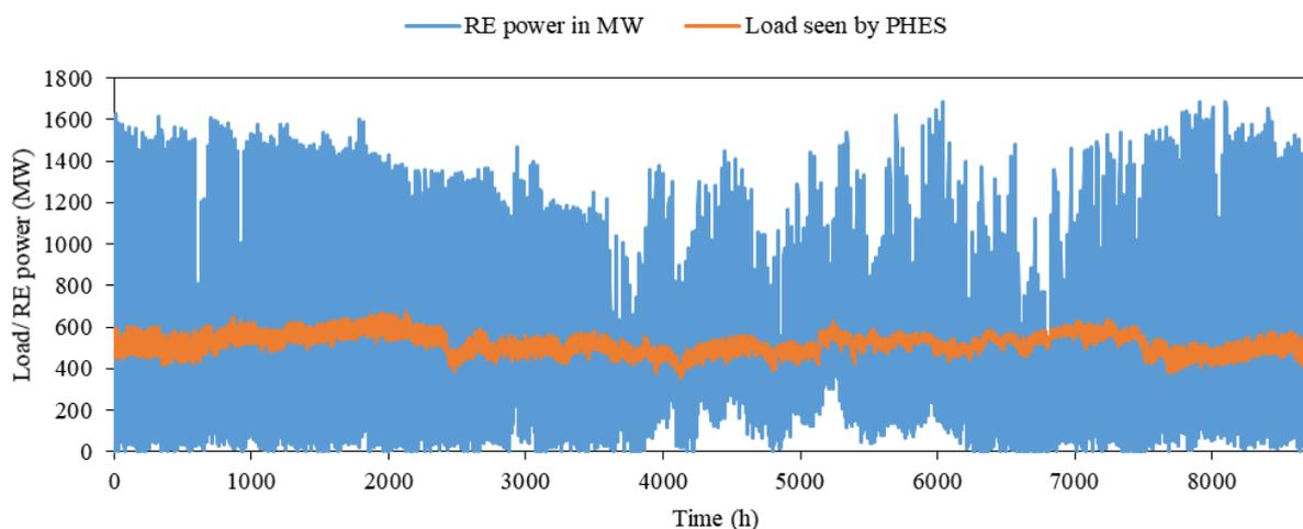
Figure 13: RE profile (both solar and wind) at the Pinnapuram RE plant and normalised load as seen by the PHEs for a year
