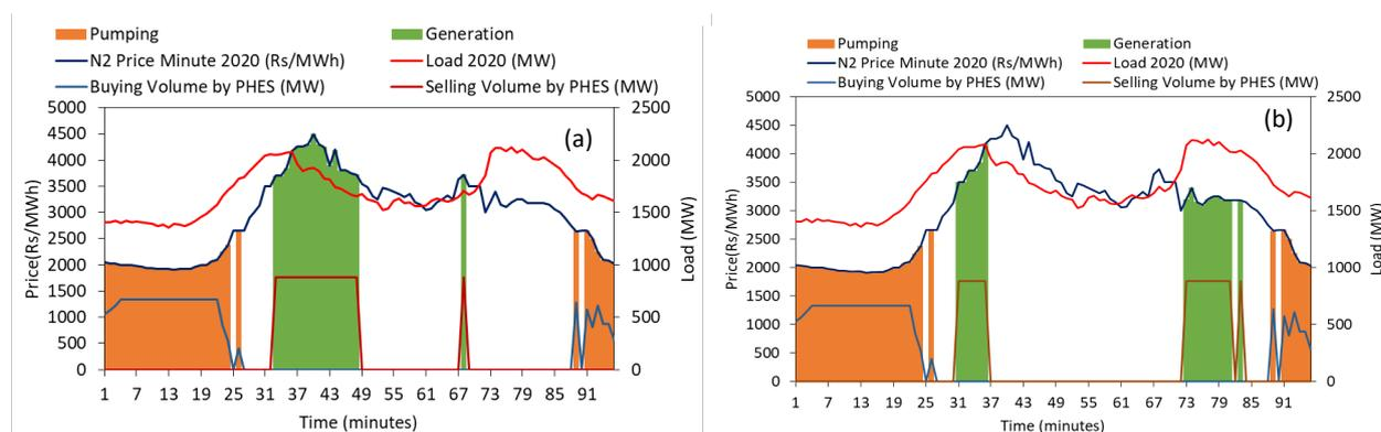
Figure 10: Dispatch plot of Tehri PHES – (a) Profit maximising; and (b) Peak-load shaving
