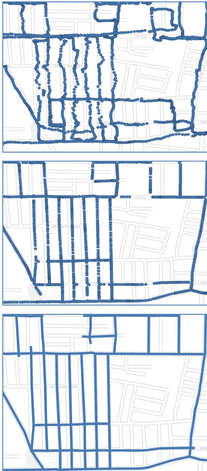
Figure 19 (top panel) Raw GPS measurements; (middle panel) snapped GPS measurements; (bottom panel) gridded road segments.
