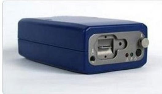
Figure 2 microAeth (model: AE51)
