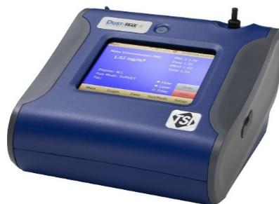
Figure 1 DustTrak aerosol monitor (model: 8530)
