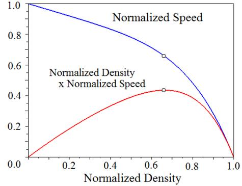
Fig 1: represents the normalized speed vs normalized density and the flow vs normalized density using the proposed power law model using  $m=0.6$  and  $n=5$ . The marked point represents the critical point where flow is at maximum.
