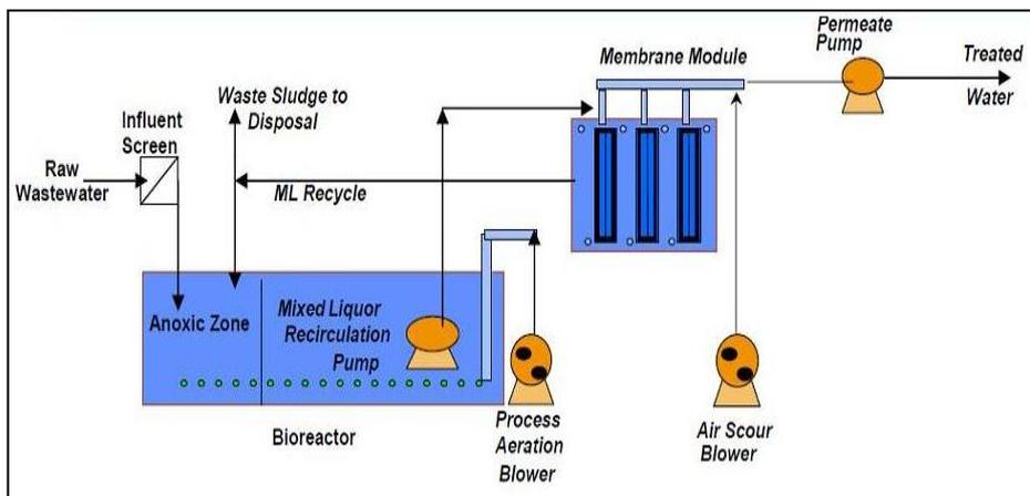
**Figure 25: Schematic View of Membrane Bioreactor**
