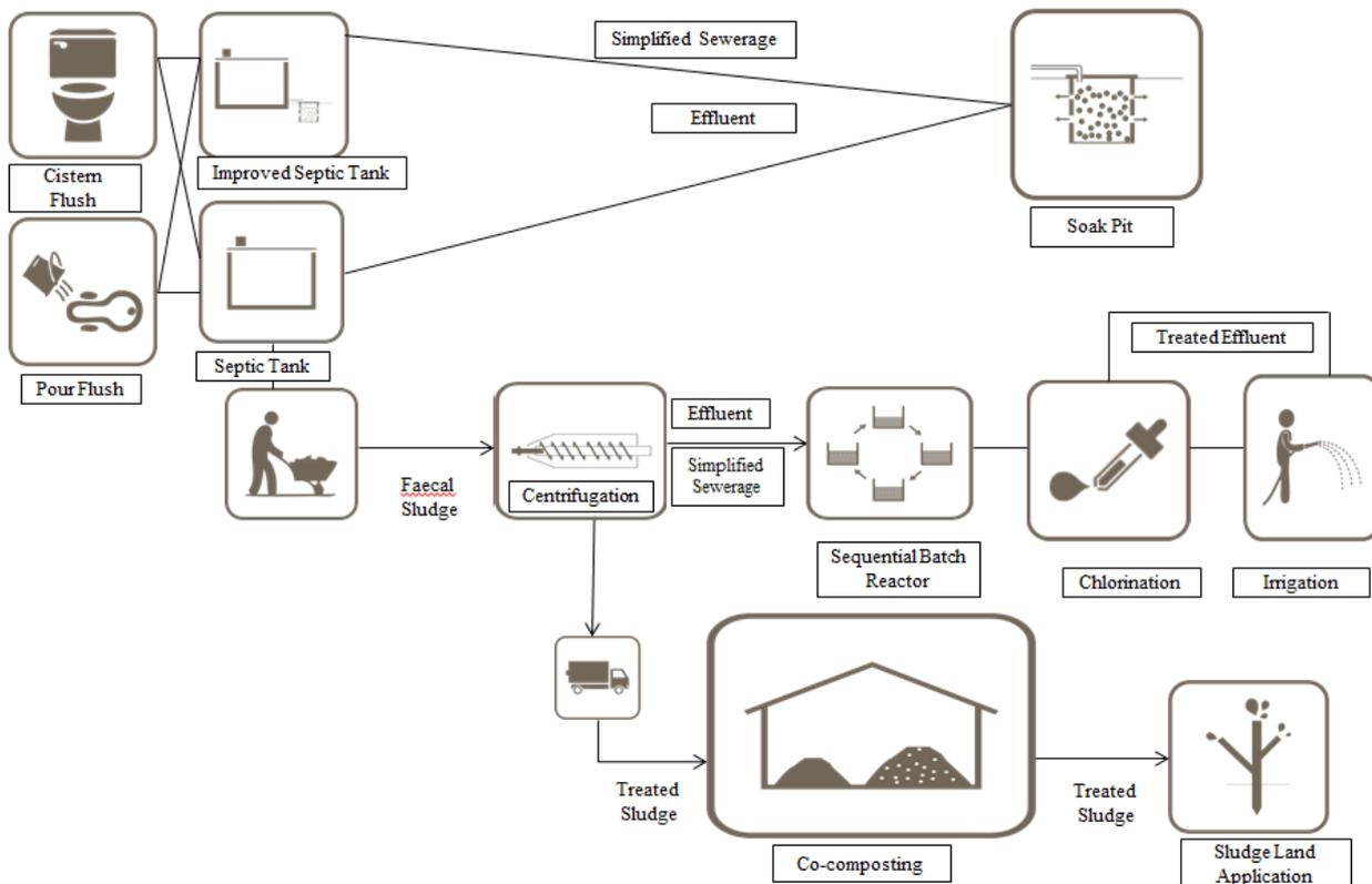
**Figure 35: Decentralised System for FSM (Centrifugation + SBR + Co-composting + Chlorination)**
