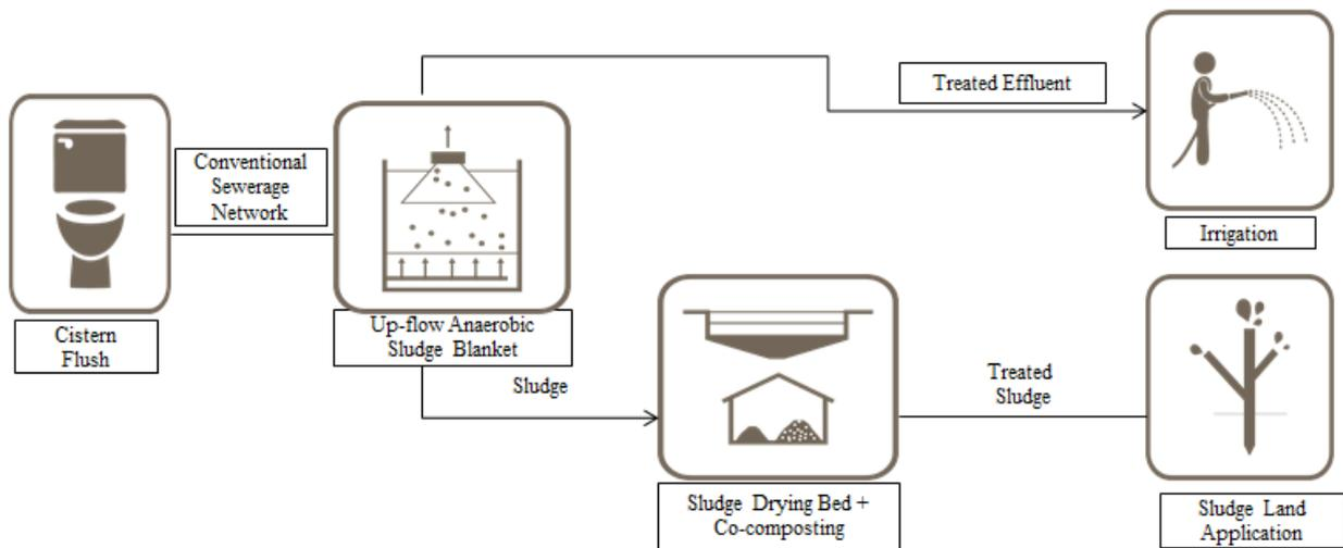
Figure 44: Networked System for FSM (UASB+ Sludge Drying Bed + Co-composting)
