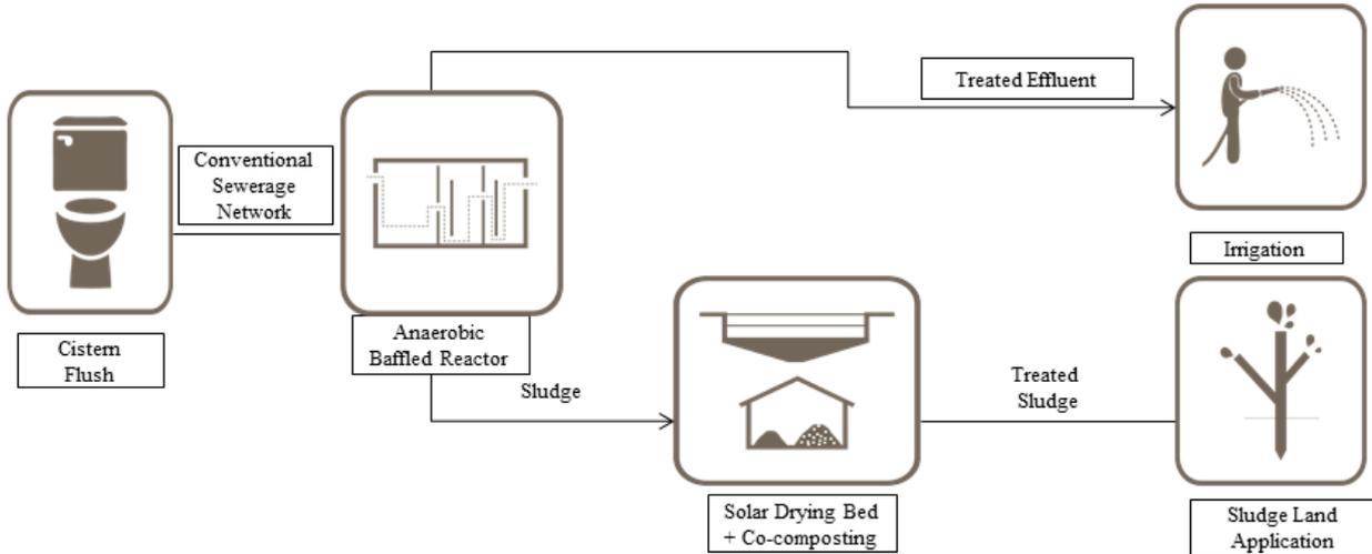
Figure 41: Networked System for FSM (ABR+ Sludge-Drying Bed + Co-composting)
