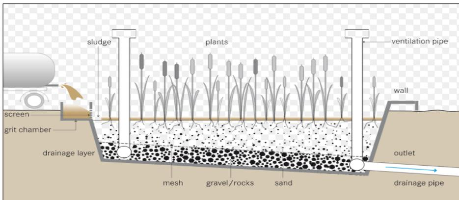
**Figure 14: Schematic View of Planted Sludge Drying Bed**
