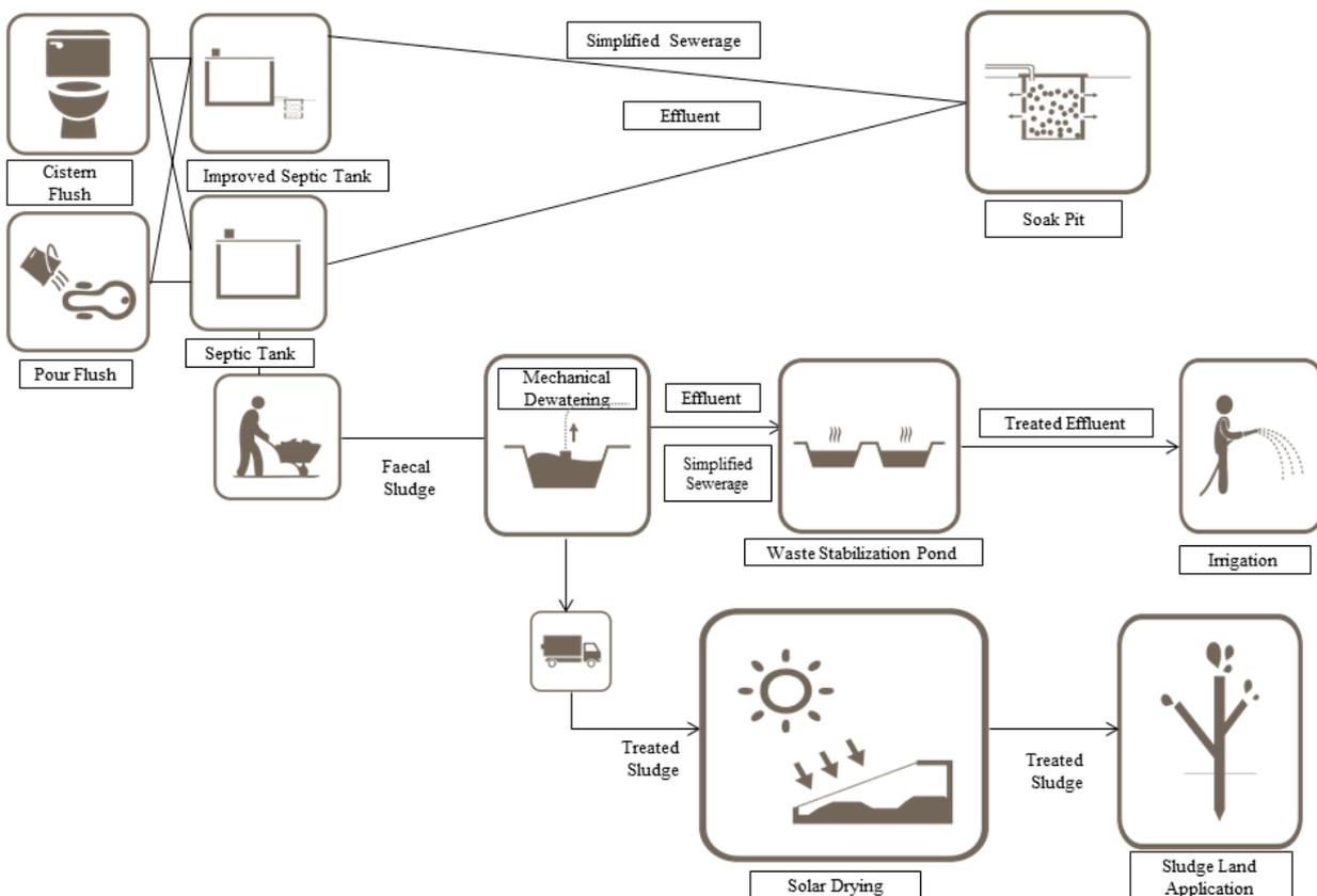
Figure 45: Decentralised System for FSM (MD + WSP + Solar Drying)
