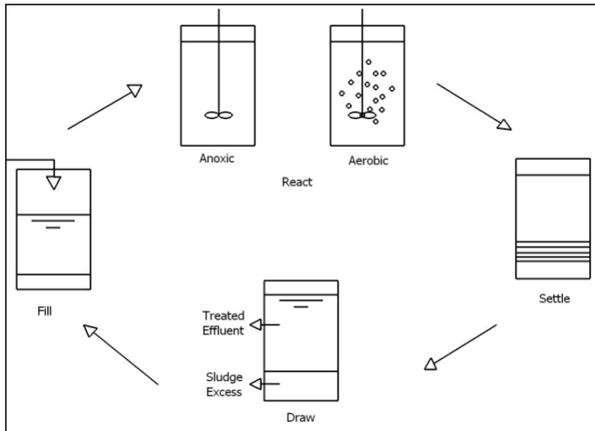
**Figure 24: Schematic View of Sequence Batch Reactor**
