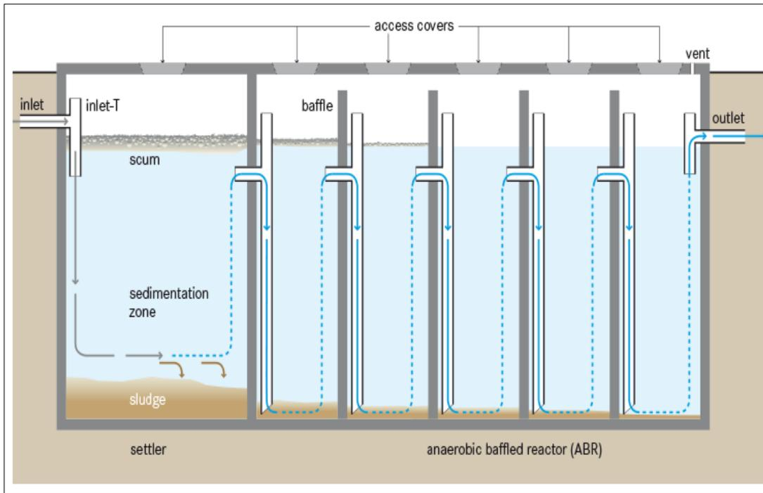
**Figure 19: Schematic View of Anaerobic Baffled Reactor**
