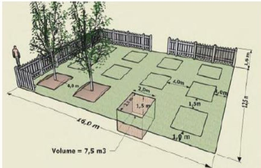
**Figure 29: Schematic View of Planted Burying Pits or Trenches**
