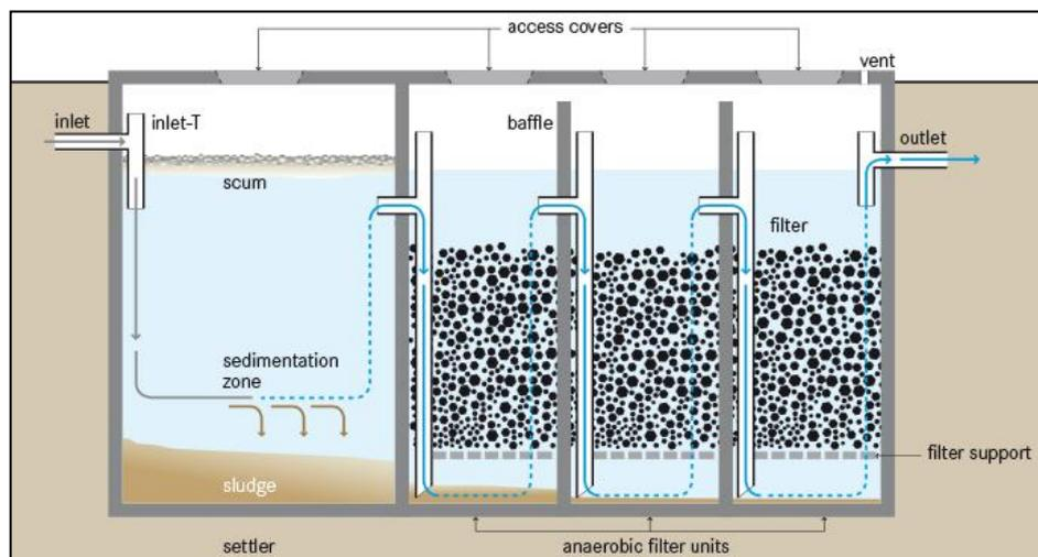
**Figure 26: Schematic View of Anaerobic filter**
