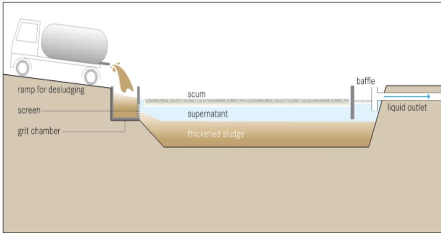
**Figure 13: Schematic View of Unplanted Sludge Drying Bed**
