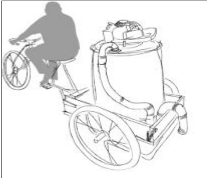
**Figure 11: Schematic of a Human-Powered FSM Transport Technology**
