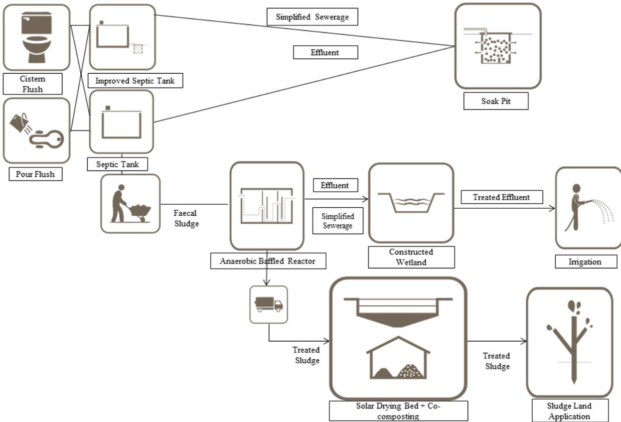
Figure 48: Decentralised System for FSM (ABR + CW + Sludge Drying Bed + Co-composting)
