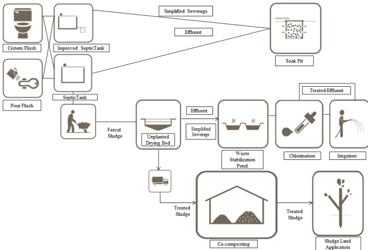
**Figure 32: Decentralised System for FSM (Septic tank + UDB + WSP + Co-composting)**
