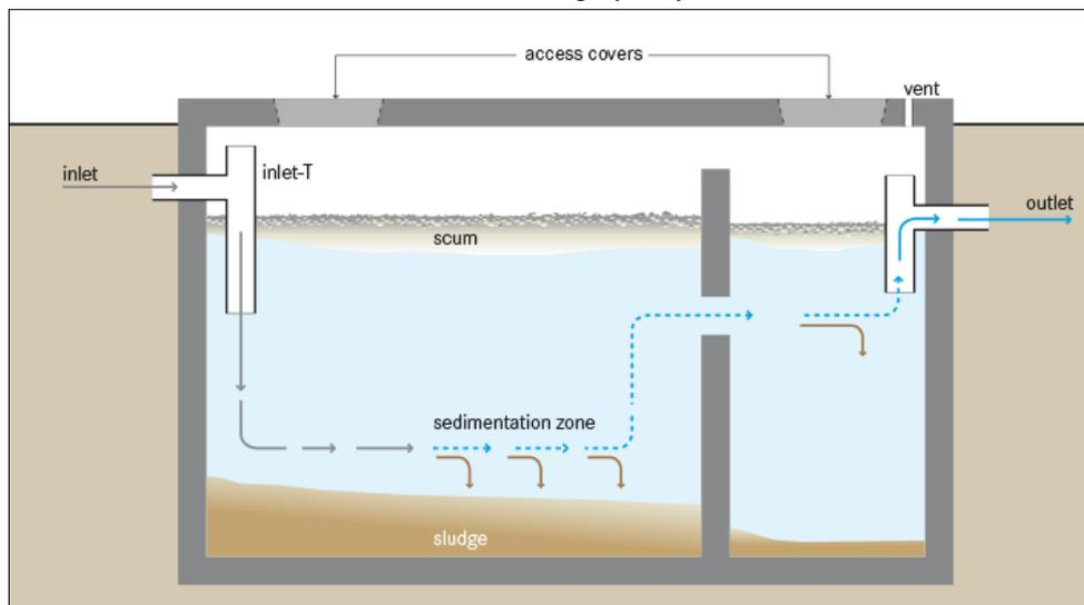
**Figure 8: Overview Scheme of a Septic Tank**
