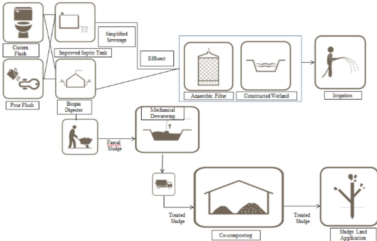
**Figure 37: Decentralised System for FSM (MD+ AF + CW + Co-composting)**
