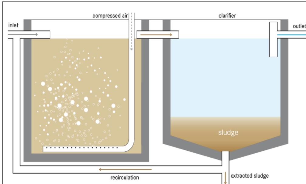
**Figure 22: Schematic View of Activated Sludge Process**
