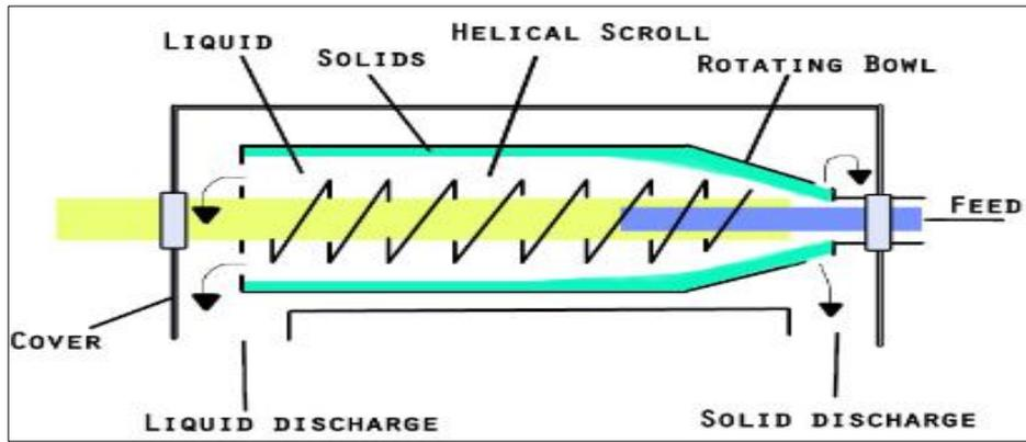
**Figure 16: Schematic View of Centrifugation**
