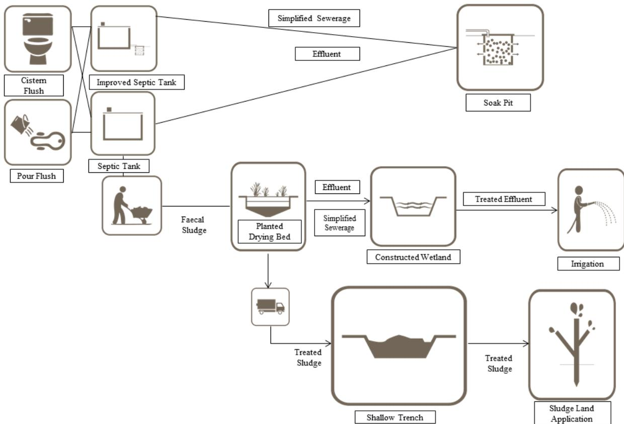
**Figure 46: Decentralised system for FSM (PDB + CW + Shallow Trenches + Chlorination)**
