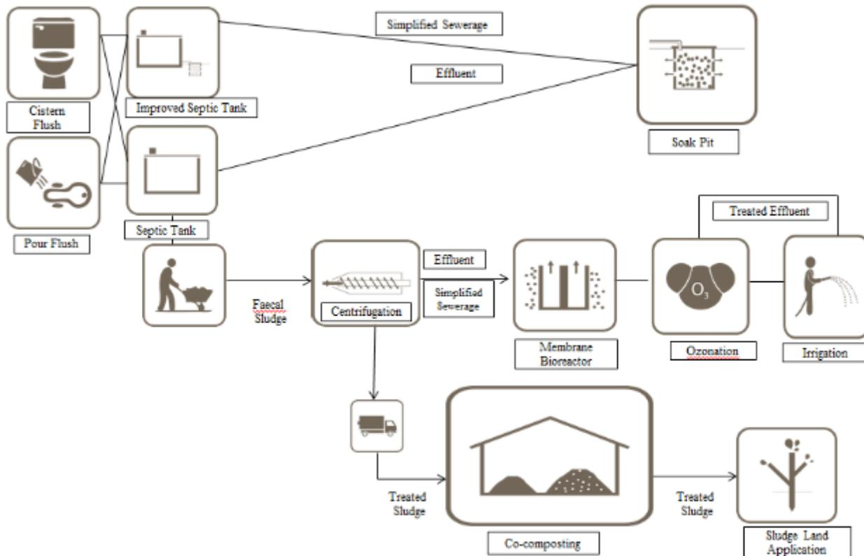
Figure 36: Decentralised System for FSM (Centrifugation + MBR + Co-composting + Ozonation)
