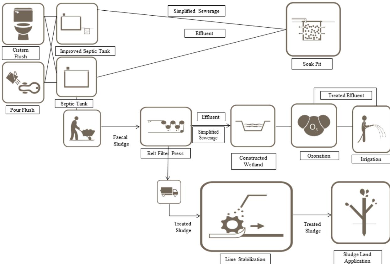
Figure 43: Decentralised System for FSM (Belt Filter Press + CW + Lime Stabilisation)
