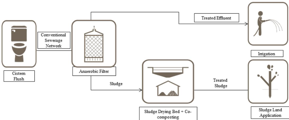
Figure 42: Networked System for FSM (AF+ Sludge Drying Bed + Co-composting)
