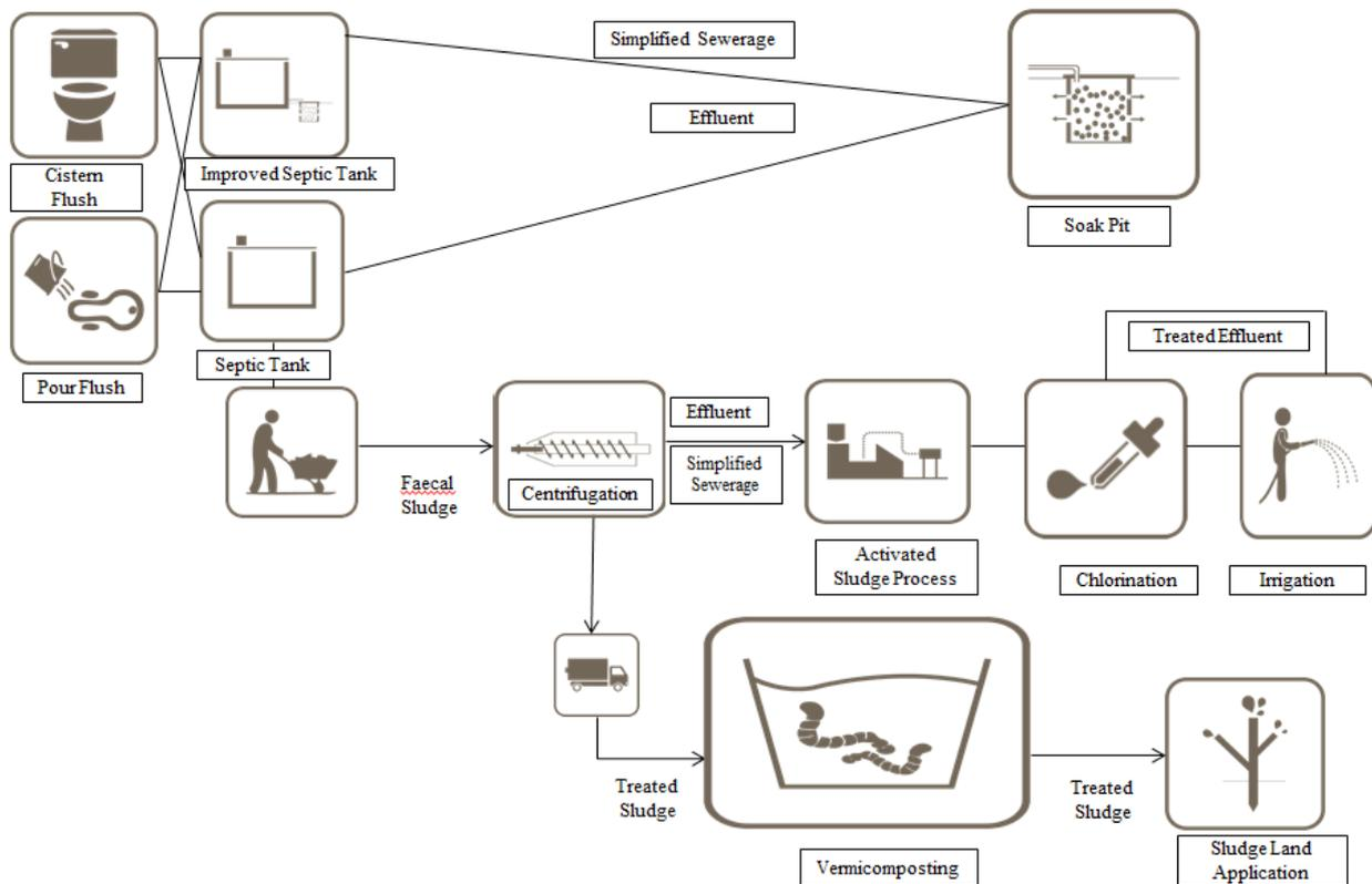
**Figure 34: Decentralised System for FSM (Centrifugation + ASP + Vermicomposting + Ozonation)**
