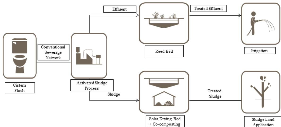
Figure 39: Networked System for FSM (ASP + Reed Bed + Sludge Drying Bed + Co-composting)
