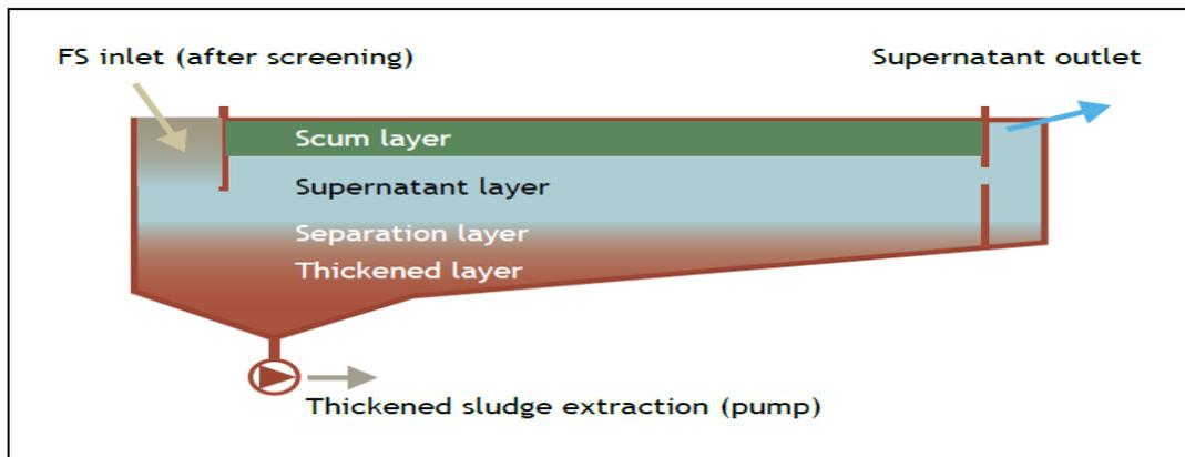
**Figure 17: Schematic View of Settling and Thickening Tank**
