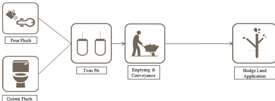
Figure 31: Twin-Pit System for FSM
