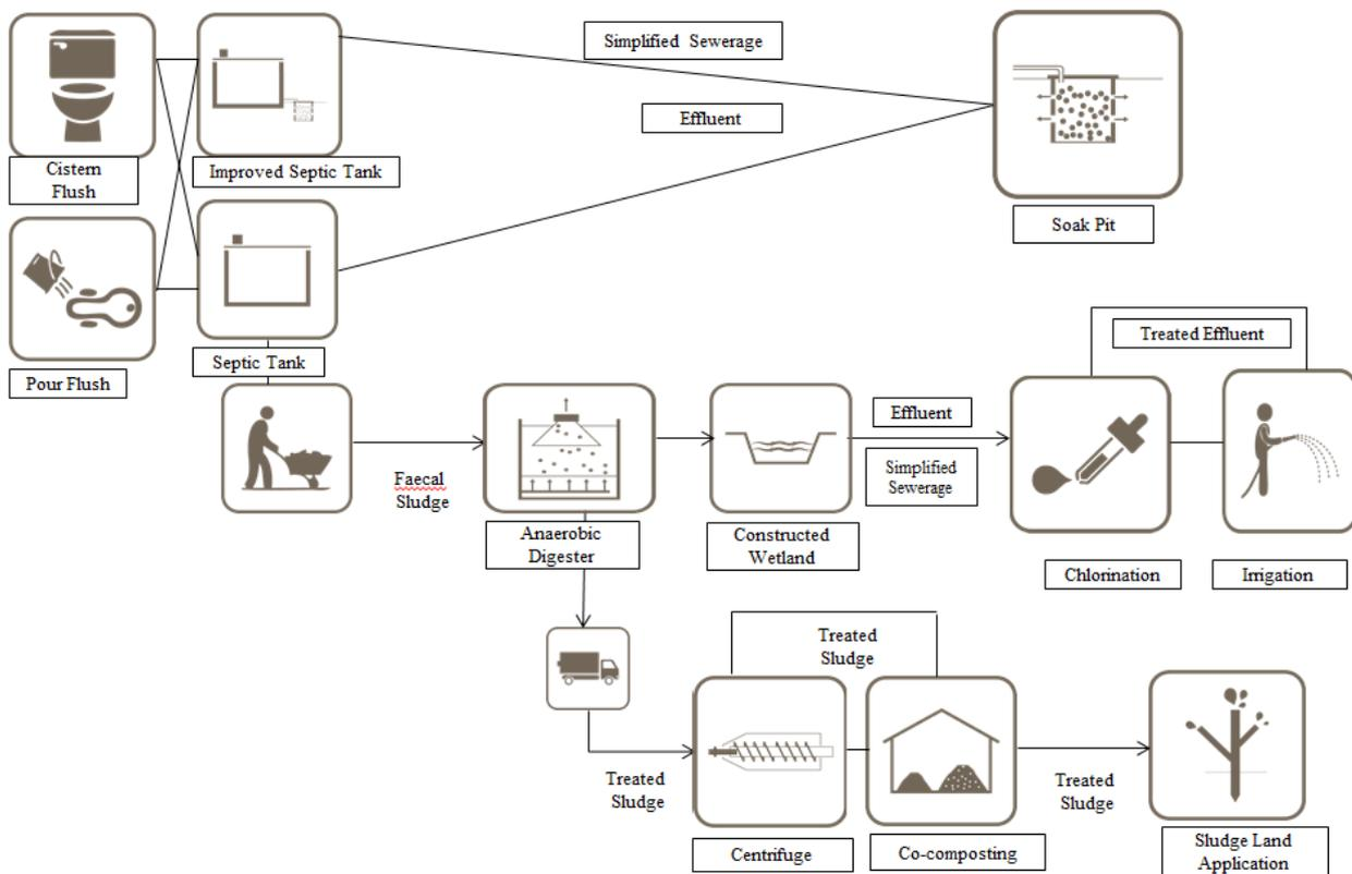
Figure 33: Decentralised System for FSM (AD + Co-composting + Chlorination)
