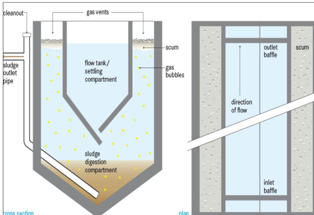
**Figure 18: Schematic View of Imhoff Tank**
