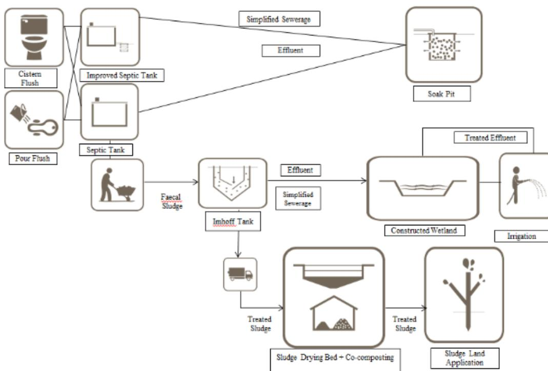
Figure 40: Decentralised System for FSM (IT + CW + Sludge Drying Bed + Co-composting)
