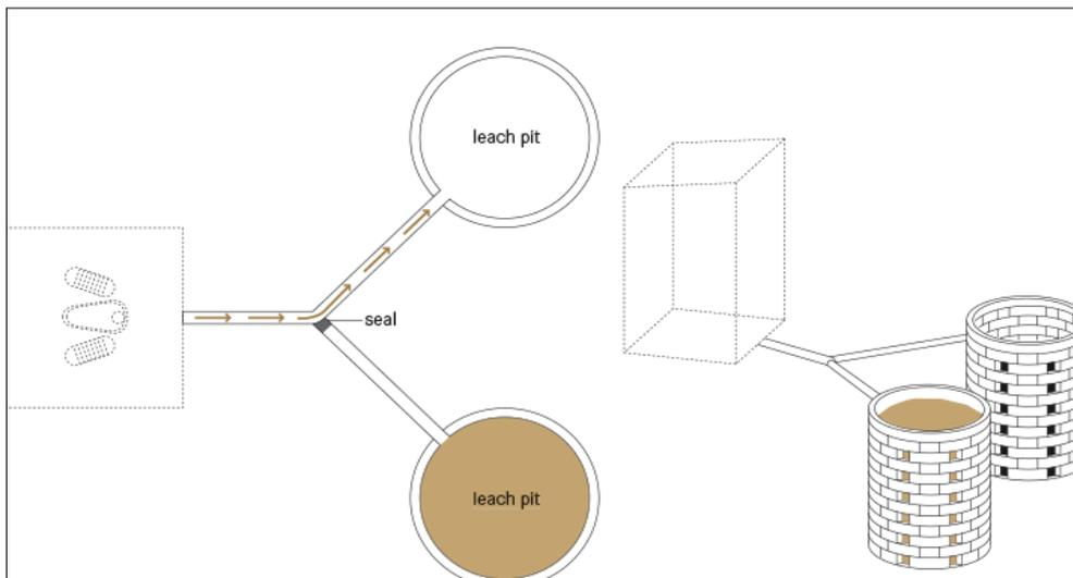
**Figure 7: A Pour Flush Toilet Linked to a Twin-Pit System**
