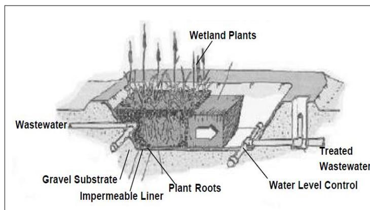
**Figure 23: Schematic View of Constructed Wetland**
