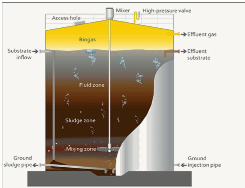
**Figure 15: Schematic View of Anaerobic Digester**
