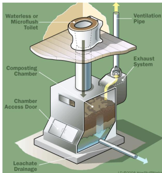
**Figure 6: Schematic View of a Composting Toilet**
