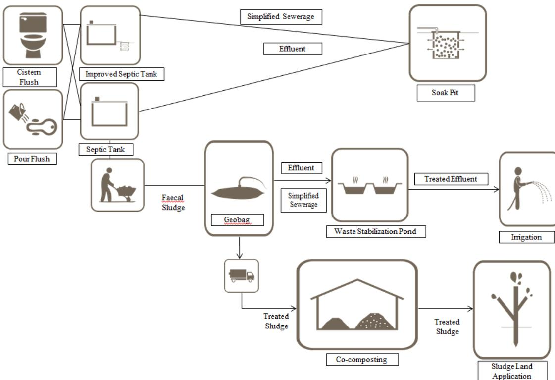
Figure 47: Decentralised System for FSM (Geobags + WSP+ Co-composting)
