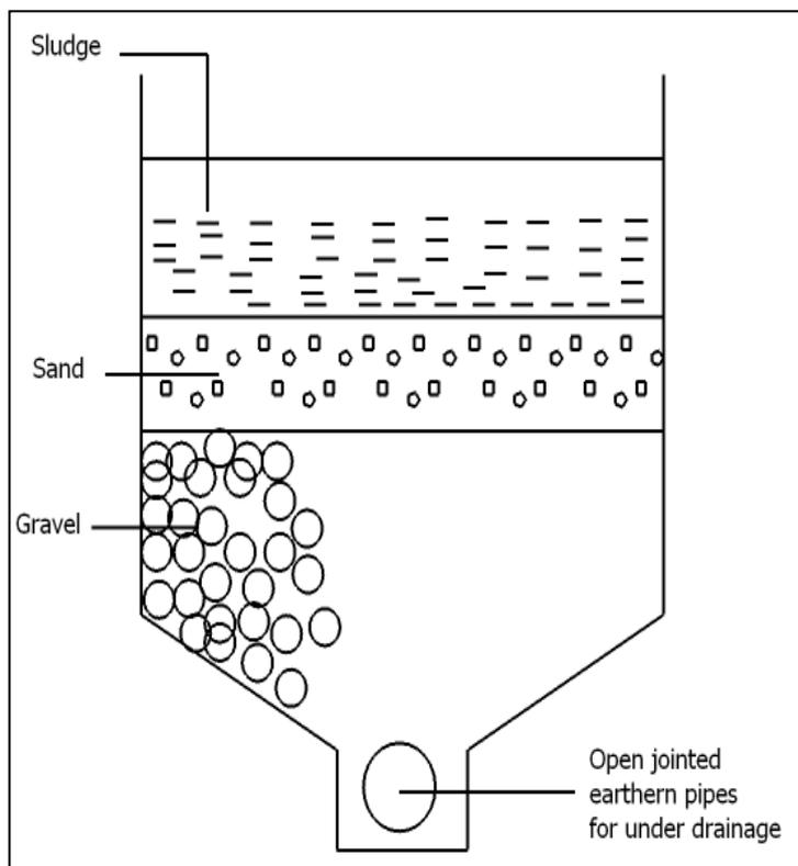
**Figure 28: Schematic View of Sludge Drying Bed**
