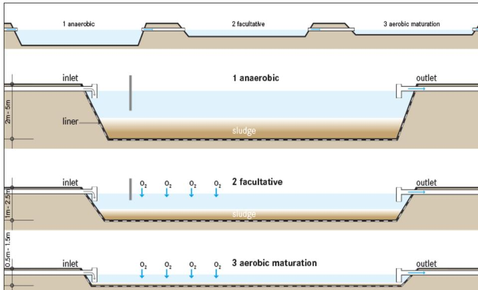
**Figure 21: Schematic View of Waste Stabilisation Pond**
