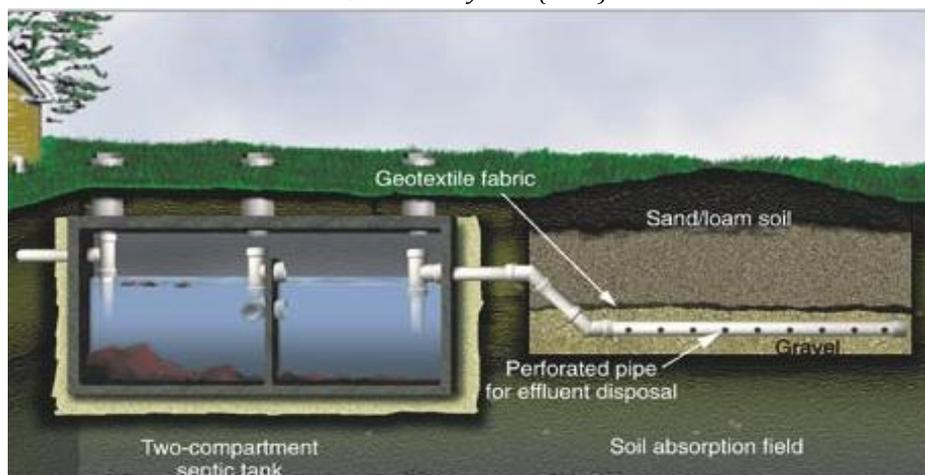
**Figure 9: Overview Scheme of an IST (Two Compartments) with a Soak Pit**
