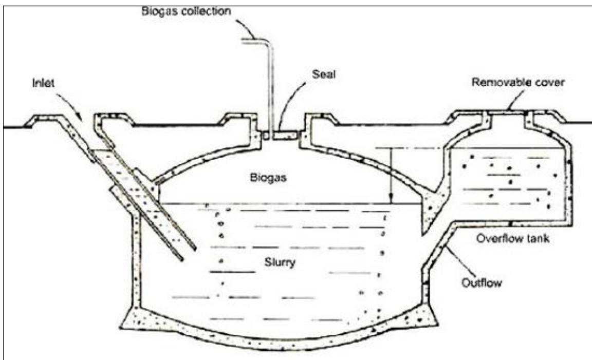
**Figure 10: Overview of a Basic Biogas Digester**
