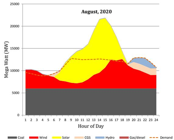
Figure 9: Projected Hourly Load Schedule for a typical day in August, 2020 (RPO trajectories)
