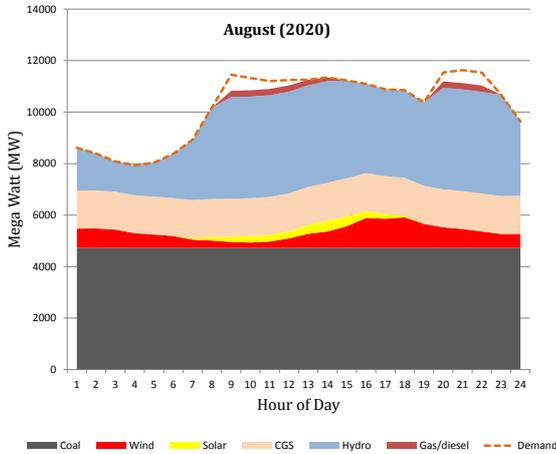
Figure 8: Projected Hourly Load Schedule for a typical day in August, 2020 (Reduced T&D losses)
