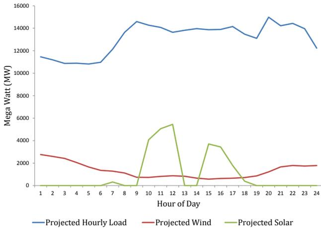
Figure 4: Projected Hourly Load vs. Projected Wind and Solar for a typical summer day in 2020
