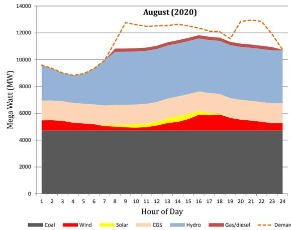
Figure 7: Projected Hourly Load Schedule for a typical day in August, 2020 (BAU)
