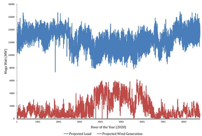
Figure 3: Projected Load vs. Projected Wind in 2020
