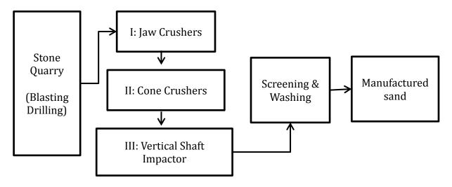
Figure 4: Manufacturing Process (Manufactured Sand)
