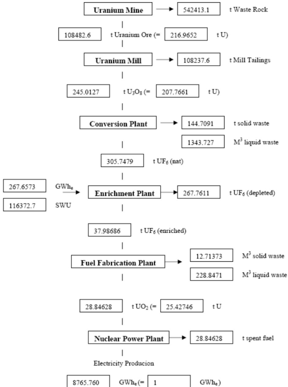
Figure 3: Nuclear Fuel Chain and Waste Production due to 1 GWh/Yr Electricity Generation
