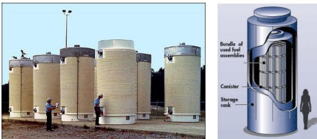
**Figure 7: Dry Cask Storage on a Concrete Pad with Cutaway Schematic of a Cask**
