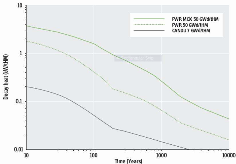
**Figure 6: Decay Heat as a Function of Time from SNF**
