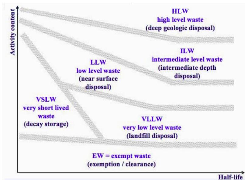
Figure 1: Conceptual Classification of Radioactive Wastes
