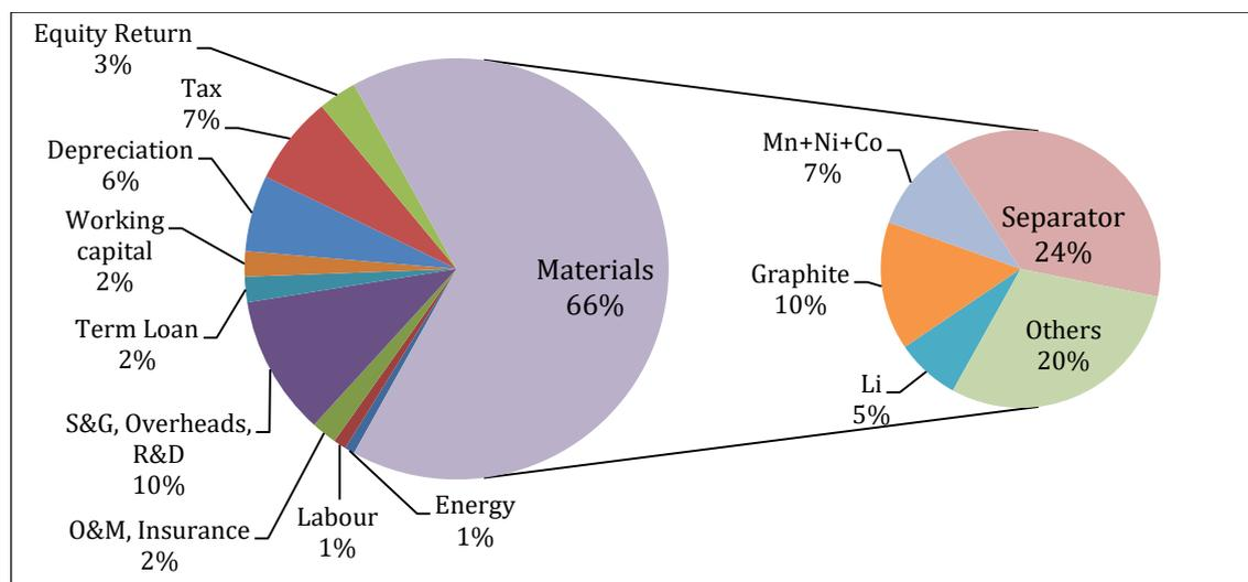
Figure 3: Cost share of various components in a LIB
