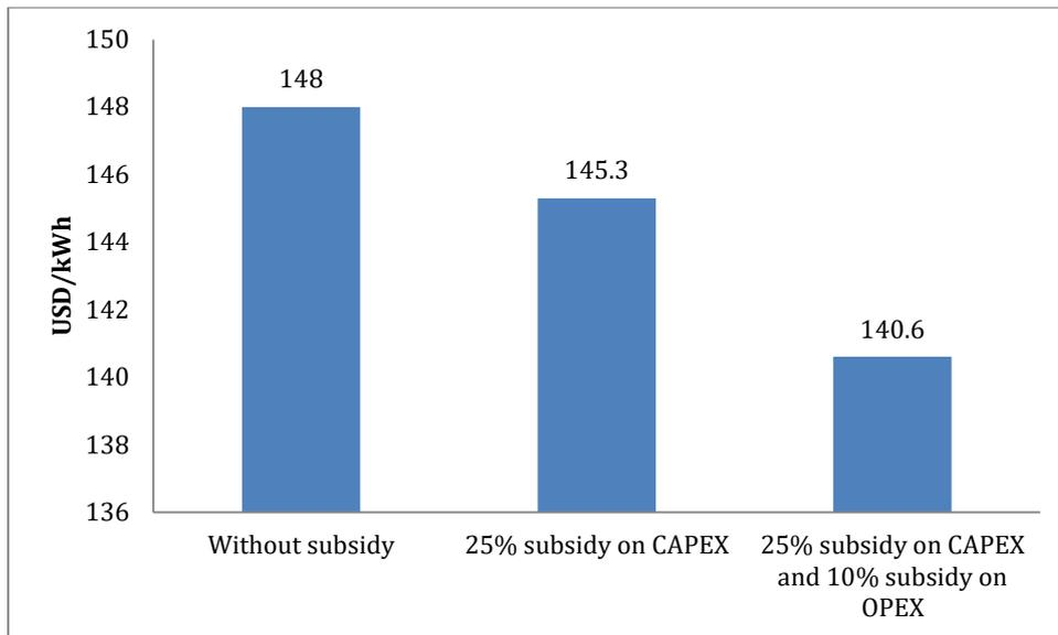
Figure 4: Impact of subsidies on LIB manufacturing costs
