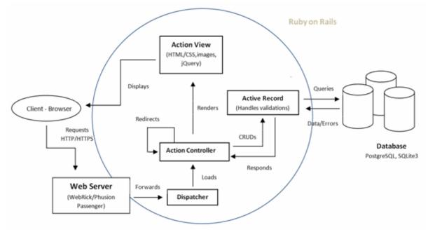
Figure 19 : Ruby on Rails – MVC Architecture
