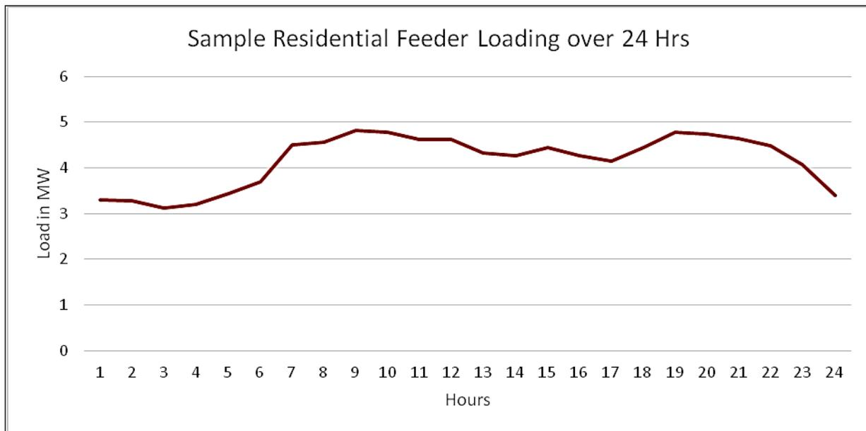
Figure 36: Electrical loading of a residential feeder (24 hours)
