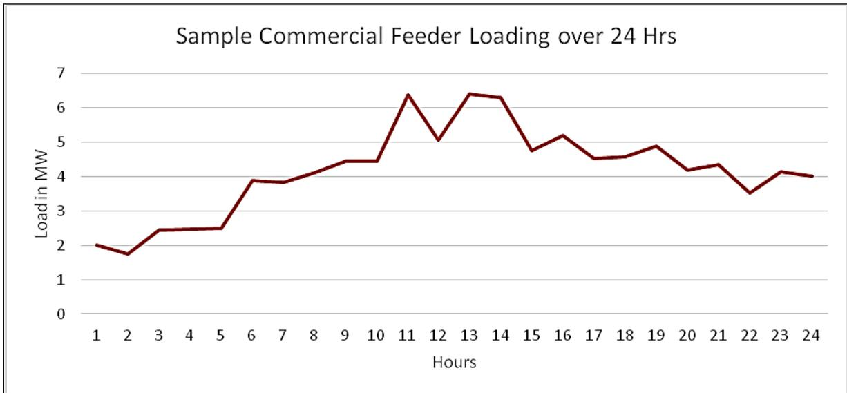
Figure 34: Electrical loading of a commercial feeder (24 hours)
