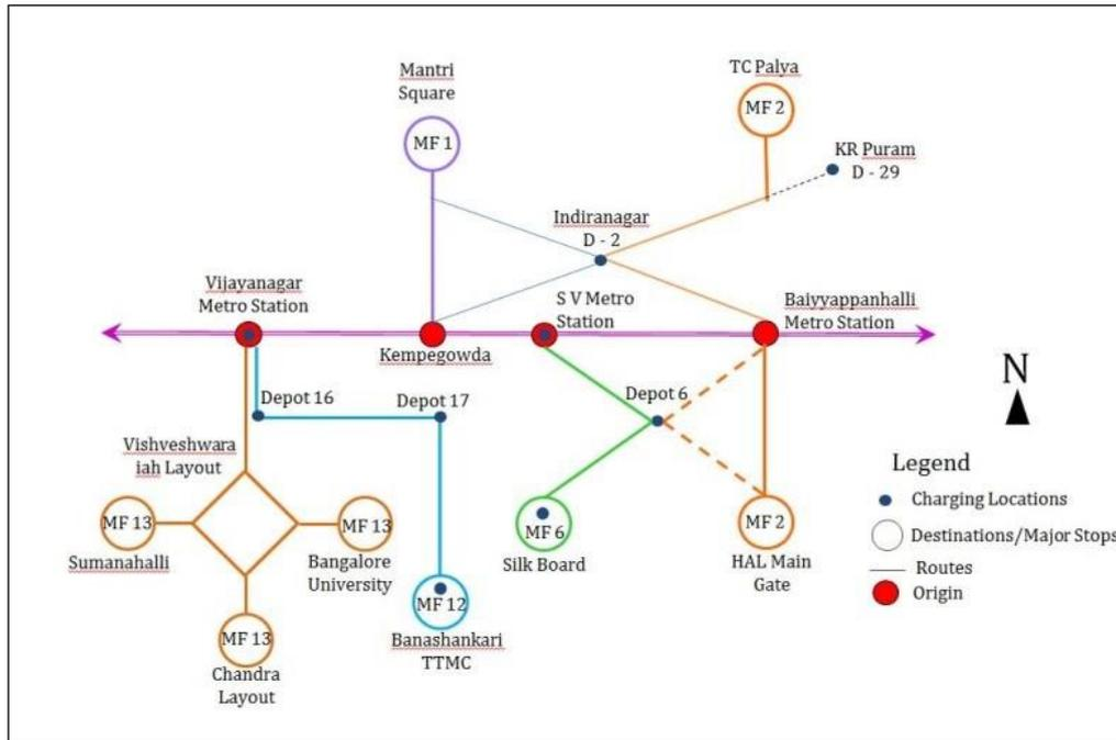
Figure 4: Feasible Metro-feeder routes with charging locations
