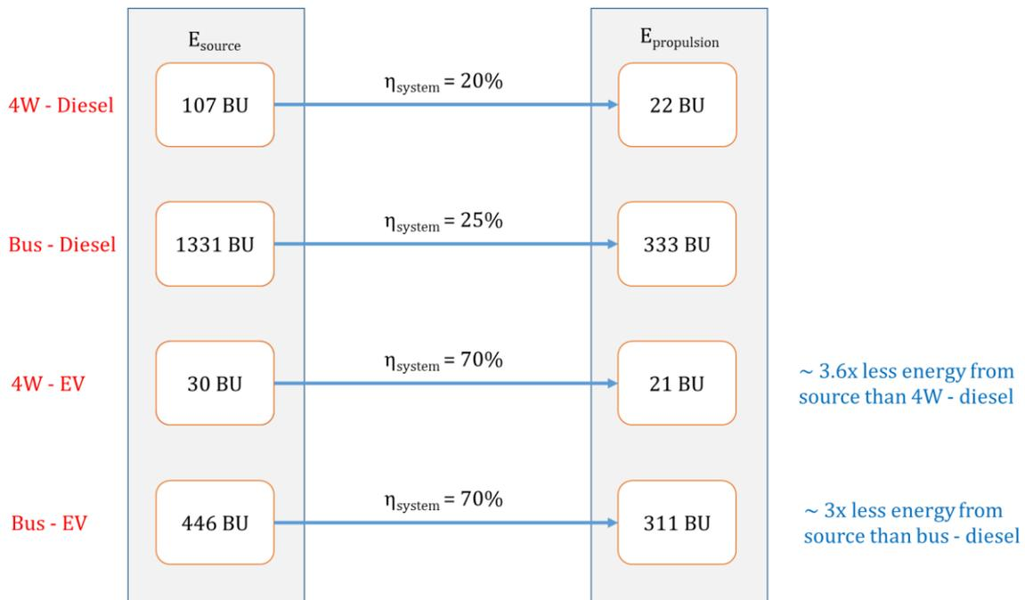
Figure 5: Flow of energy requirements from source to wheel/propulsion
