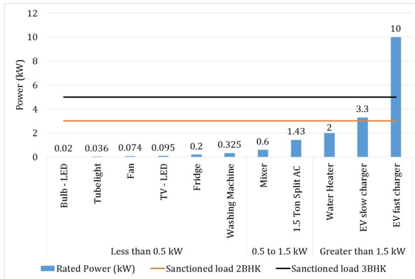
Figure 20: Comparison of power rating of typical equipment<sup>22</sup>
