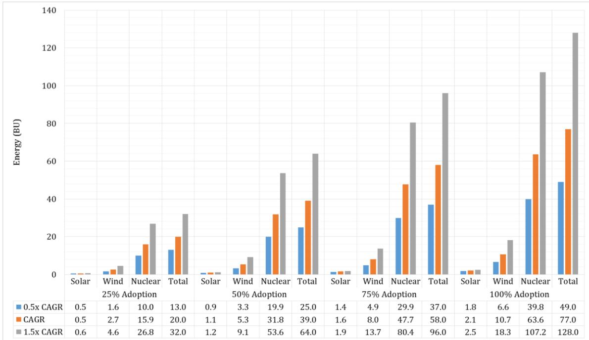
Figure 18: Contribution of energy needs from different fossil-free energy sources for 2030
