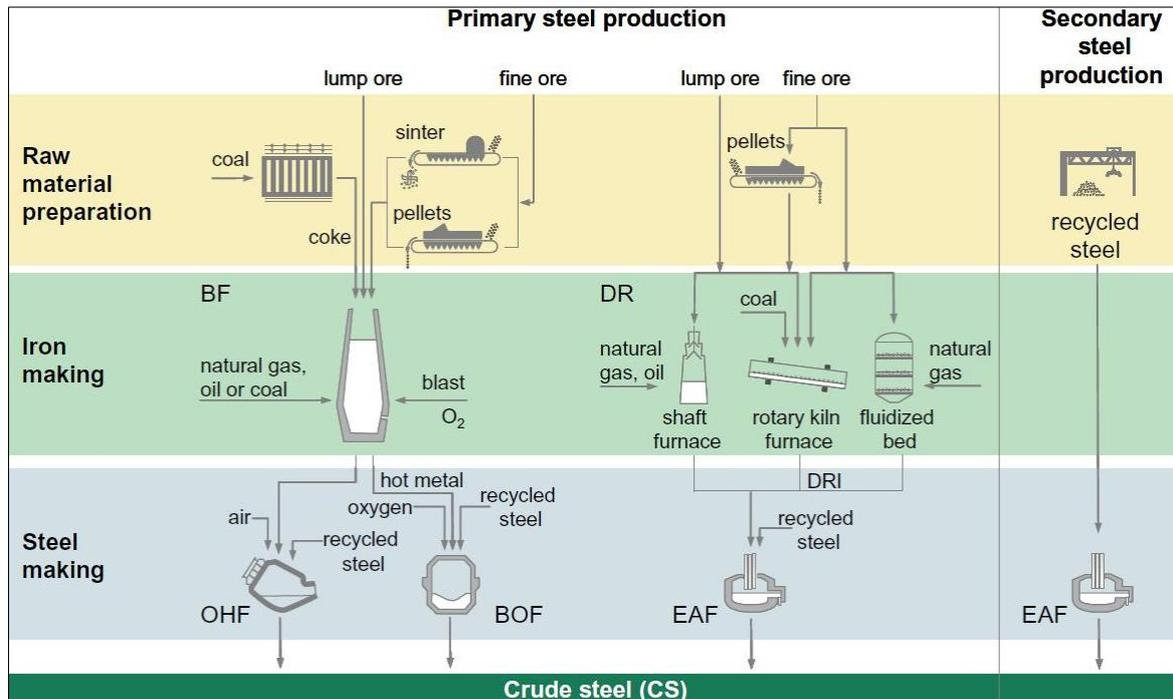
Figure 11 Iron and Steel Production Process routes (17)
