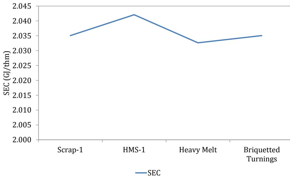
Figure 40: SEC of different scrap types
