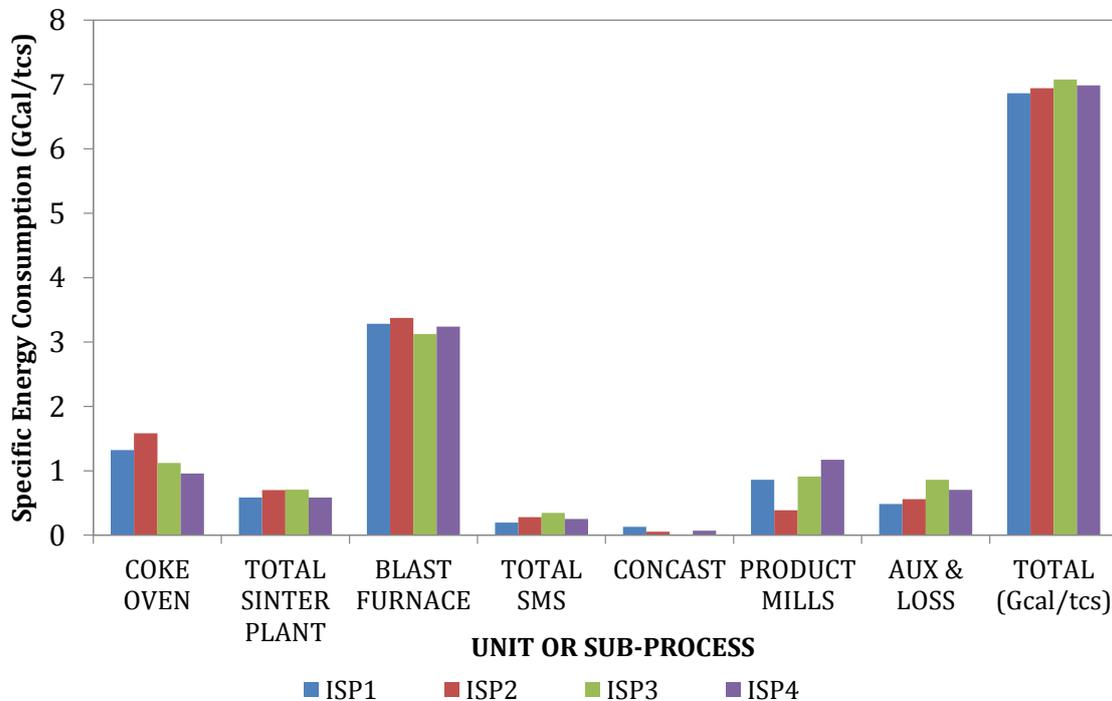
Figure 48: Energy Balance Comparison for Sample ISP Plants
