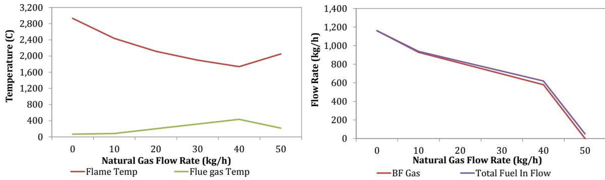
Figure 23: Hot Stove Performance with Mixed Fuel Injection
