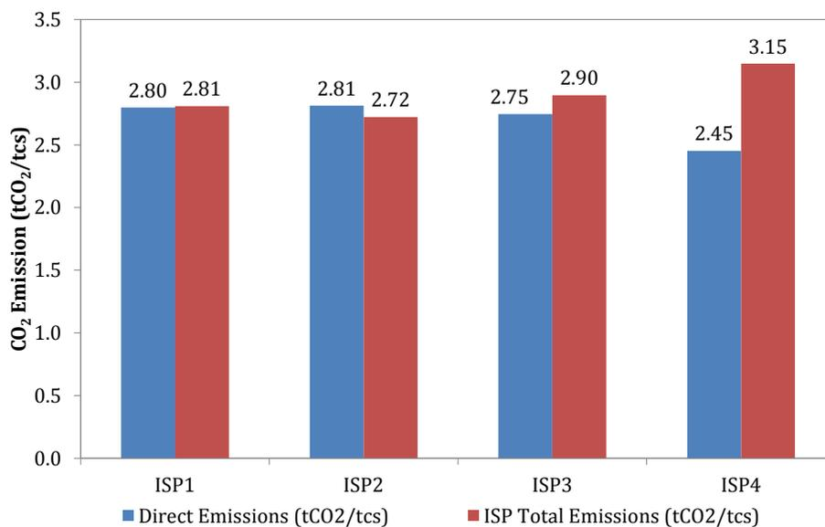
Figure 50: CO<sub>2</sub> Emission Comparison of Sample ISP Plants
