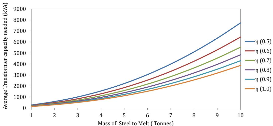
Figure 44: Sensitivity analysis for estimating the transformer capacity
