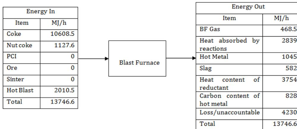
Figure 13: Energy Balance of Blast Furnace with Coke Input
