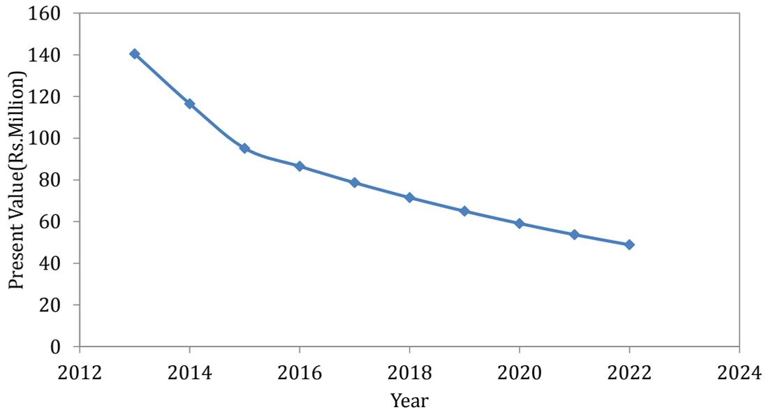
Figure 76: Present value of annual energy savings for Injection of coke oven gas in BF
