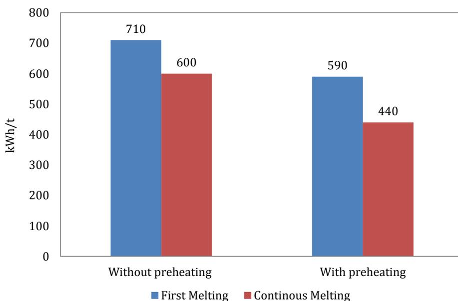
Figure 46: Comparison of equipment with and without preheating
