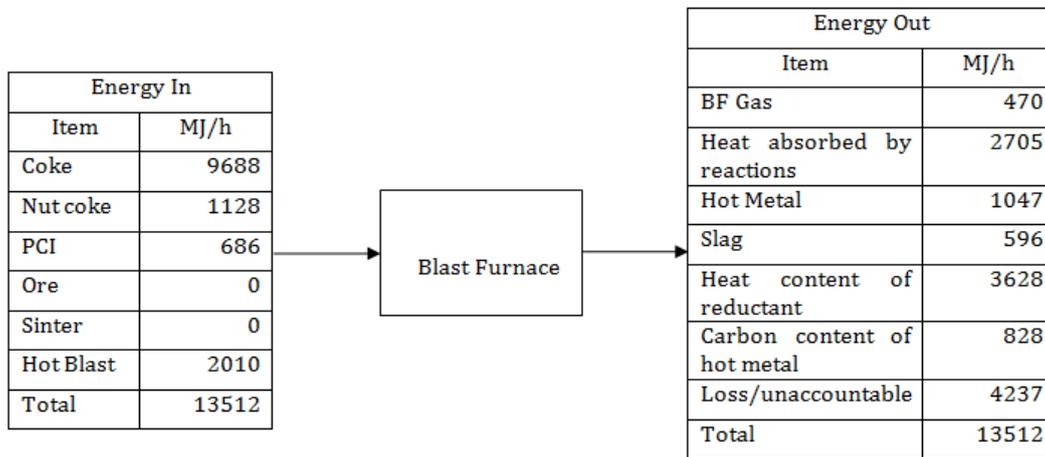
Figure 15: Energy Balance of Blast Furnace with Coke and PCI Input
