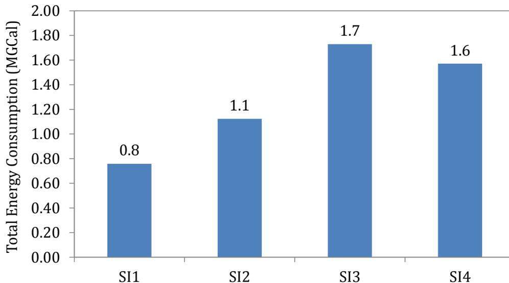
Figure 66: Thermal energy consumption across sample SI plants
