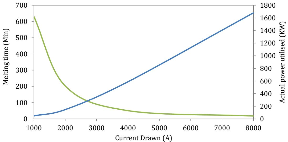
Figure 43: Performance of the furnace with respect to melting time and power utilised with increasing current drawn from the transformer
