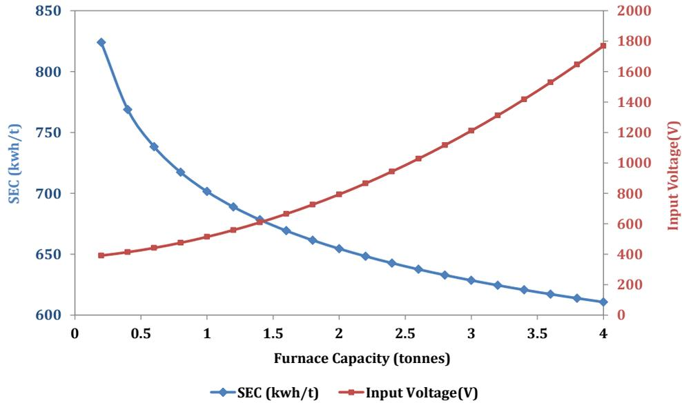
Figure 41: Energy consumption behaviour with increasing furnace capacity and input voltage
