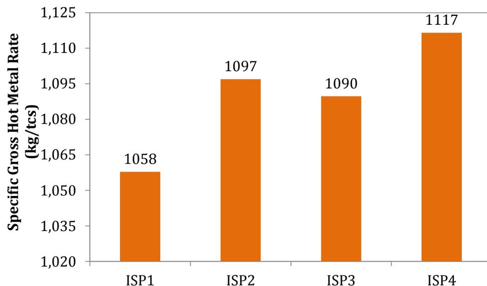
Figure 56: Specific Gross Hot Metal Consumption for Sample ISP Plants
