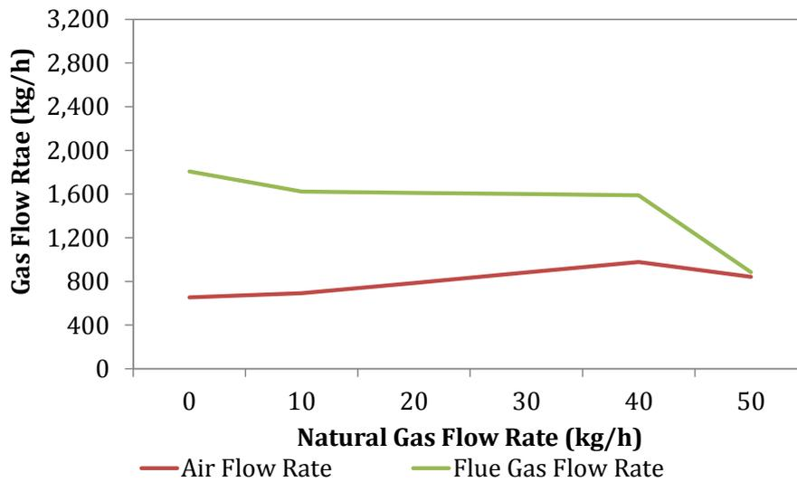
Figure 24: Hot Stove Performance with Mixed Fuel Injection
