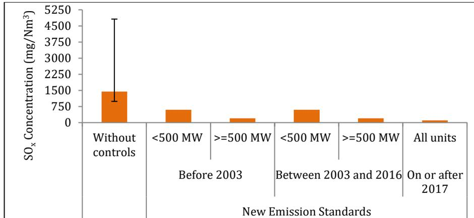
Figure 1: Current concentrations and targeted concentration of SO<sub>x</sub> in flue gas<sup>2</sup>
