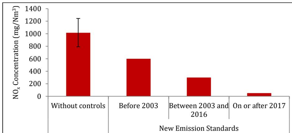
Figure 2: Current concentrations and targeted concentration of NO<sub>x</sub> in flue gas
