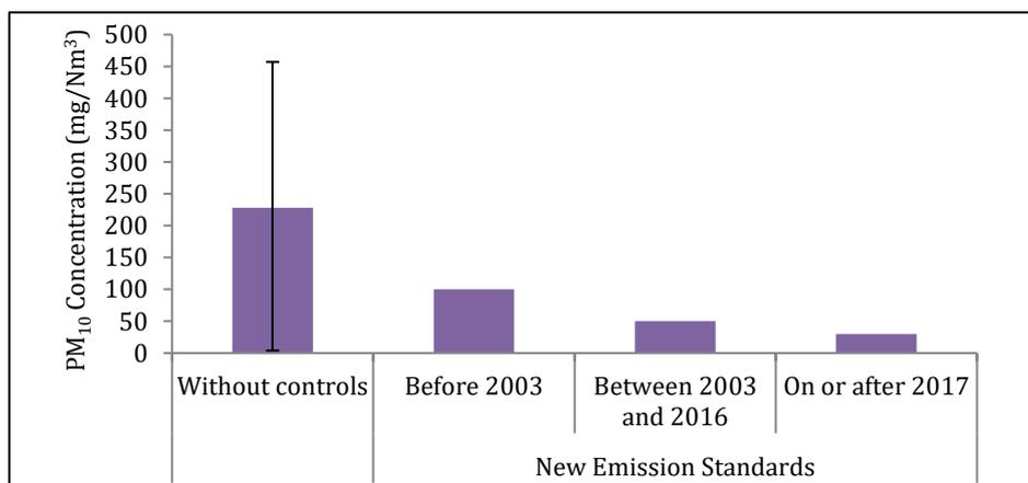
Figure 3: Current concentrations and targeted concentration of PM<sub>10</sub> in flue gas
