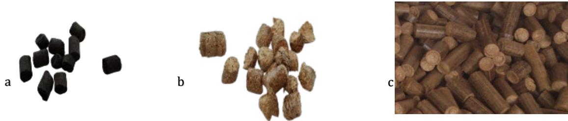
Figure 7: Various forms of processed biomass: a) torrefied pellets, b) pellets, and c) briquettes
