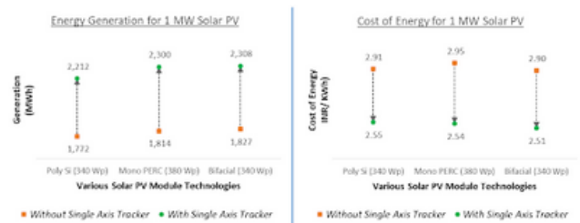
Figure 3: Generation and cost of energy profiles for 1 MW solar-PV system with and without single-axis tracking system
