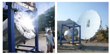
Figure 2.21: Cast iron core cavity receiver and Scheffler dish
