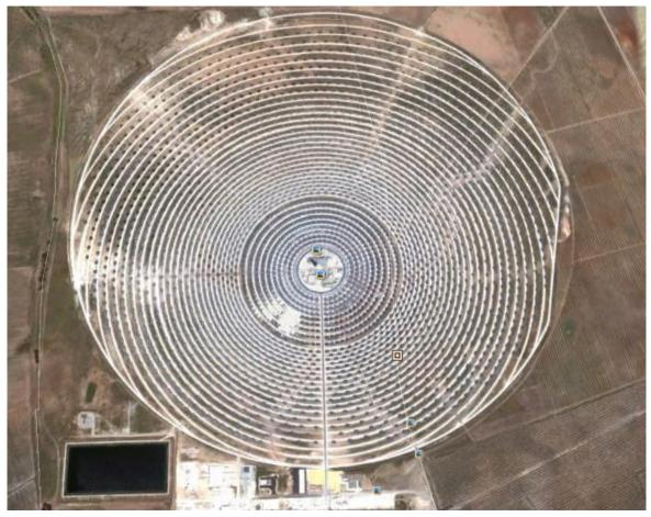
Figure 2.8: Heliostat field at Gemasolar, Spain
