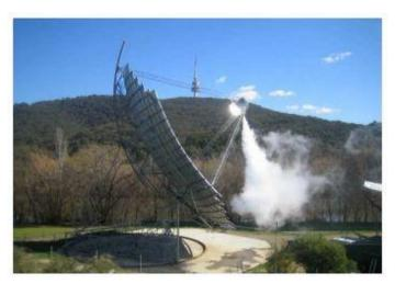
Figure 2.22: The SG4 dish in testing for the direct steam generation
